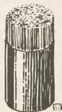
FIG. 32.—Method of securing a number of short lengths of wire in order to make the ends square.
