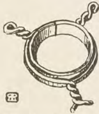
FIG. 33.—Method of using iron binding wire.
