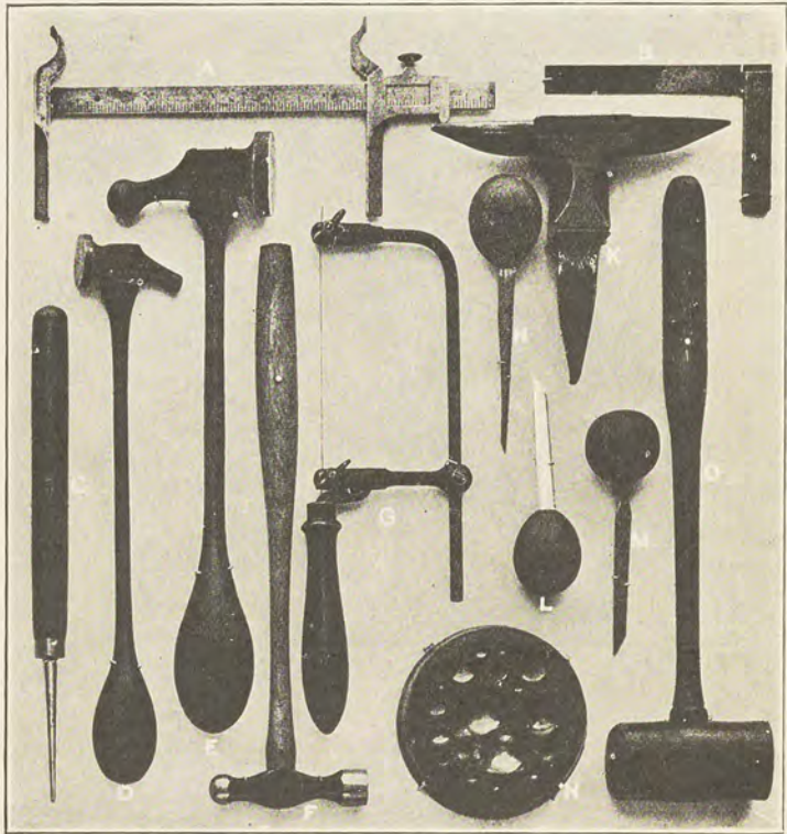
FIG. 29.—A. Sliding callipers, or slide gauge. B. Steel square. C. Straight steel burnisher. D. Small repoussé (or chaser's hammer). E. Large repoussé (or chaser's) hammer. F. Jeweller's hammer. G. Jeweller's piercing saw. H. Spitsicker. K. Sparrowhawk. L. Bullsticker. M. Flat scorper. N. Lead cake. O. Horn mallet.
