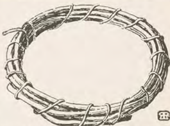
FIG. 17.—A hank of wire, secured with iron binding wire, ready for annealing.
