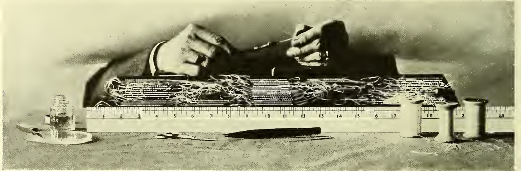
Stringing a pearl collar in sections; cleaning and reaming out a pearl
