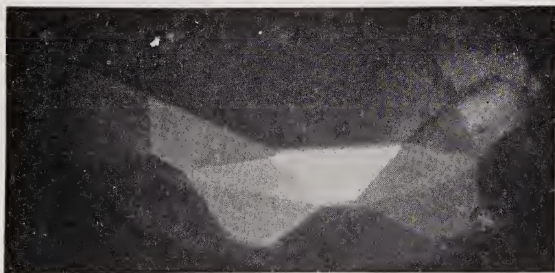
Figure 100 Garnet-and-glass doublet under 30X. Note the sharp luster change on bezel facets.
