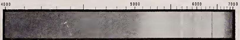
Diamond — treated pink (orange fluorescence). Line at 5700 Å is a fluorescent line * * *
