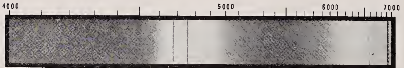
Corundum — Ruby and synthetic ruby, purple sapphire and dark padparadscha (direct transmitted light) * * *
