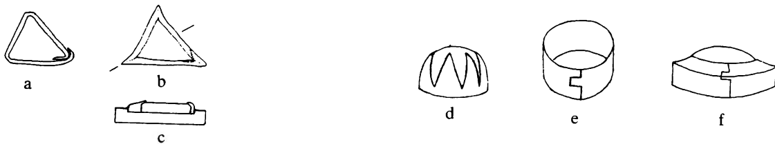
Fig. 84. Less common variations on band settings. a-c) A pinched setting (2b), with the overlapping bands of the collet (a), pinched corners (b) and a section (c). d) Star setting. e-f) Shoulder setting, different stages.
