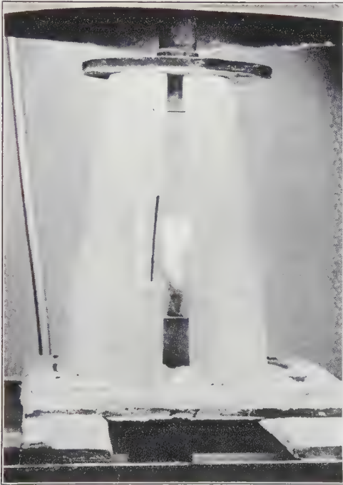
Fig. 103 Verneuil Furnace for Manufacture of Synthetic Corundum
