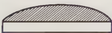
An opal doublet with a thin top section of precious opal attached to a base of common opal
