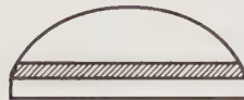
An opal triplet, which is the opal doublet with a cap of quartz
