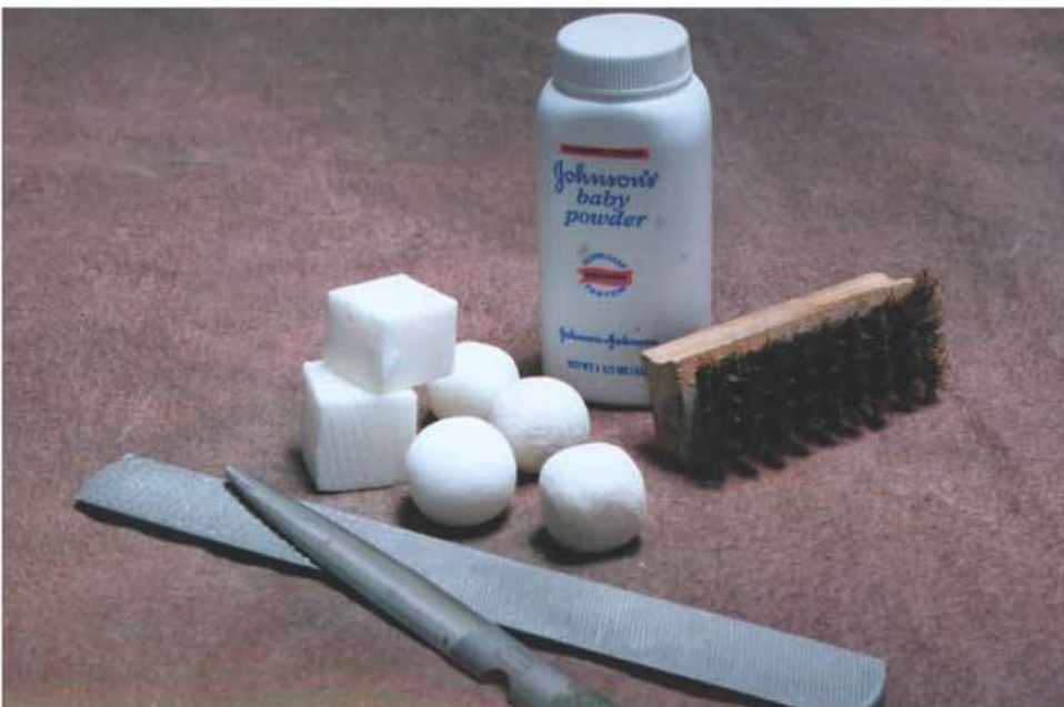
Use the rasp and wax file to shape the white wax. Baby powder and a wire brush help clean shavings from the files.
