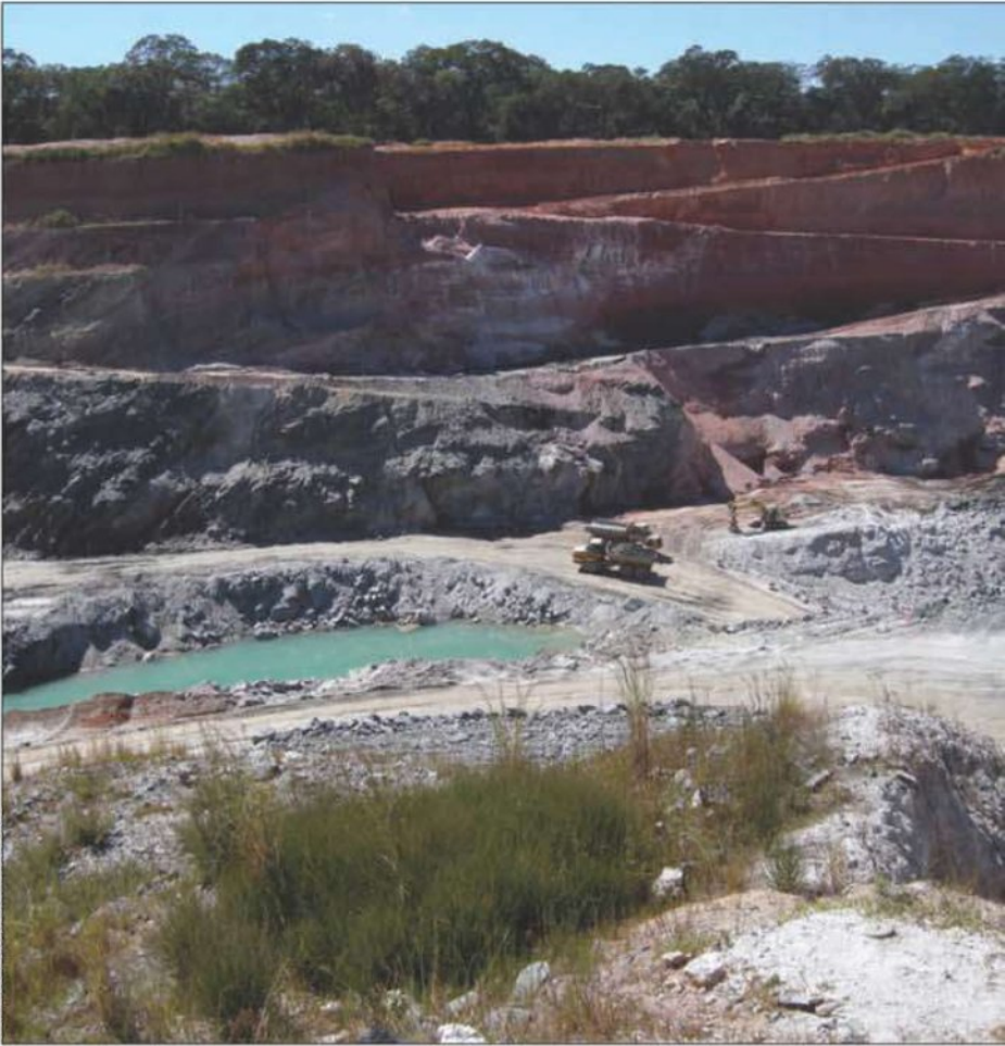
A large haul truck passes by one of the water-filled pits that are created as the emerald-bearing reaction zones are mined out.
