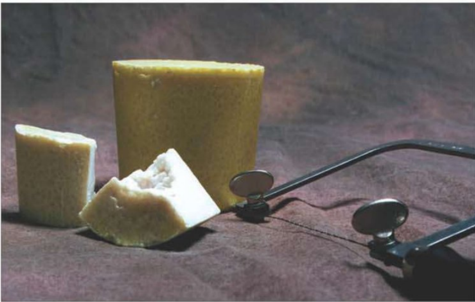
The file-like cut of the spiral wax blade easily gets through the off-white glaze that protects the white water wax.
