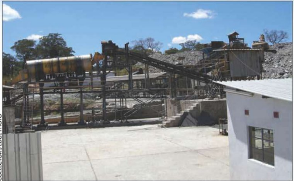
The primary washing and sorting station for emerald rough utilizes a rotating trommel drum to separate the gem material from the days and mica.
