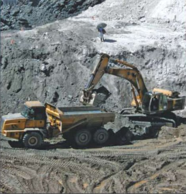
Heavy equipment such as this excavator and haul truck are used to move the enormous tonnages of waste rock generated in the search for the gem-quality emeralds.
