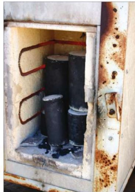
Once the flasks are stacked in the kiln, the kiln is brought up to about 1,400 degrees F.
