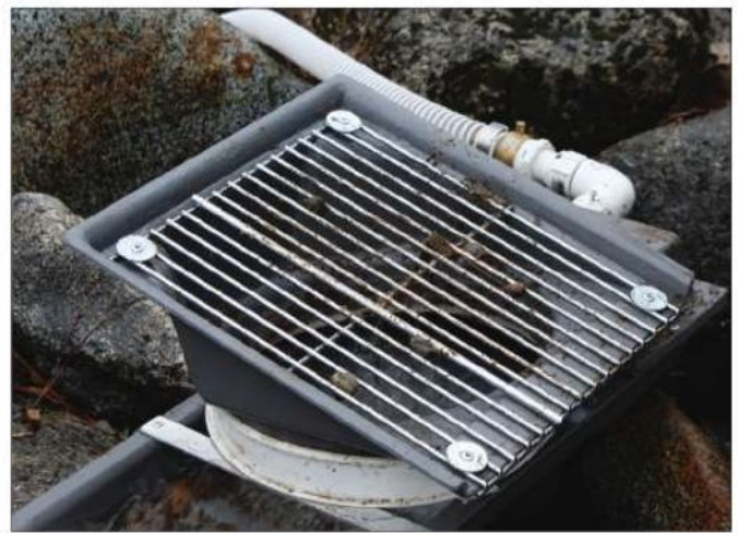
A ring was cut from the top of a 5-gallon plastic bucket and used to attach a grizzly to this power sluice.
