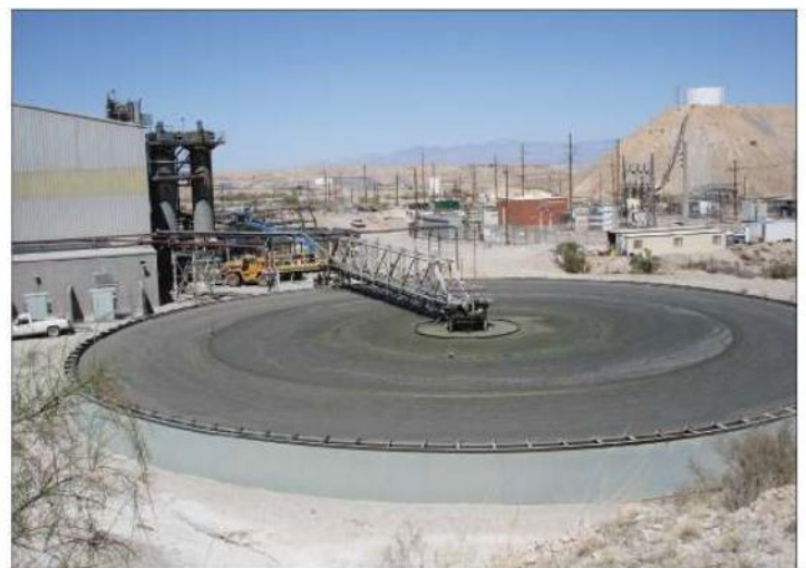
In the Asarco Mission mine's concentration tanks, a slurry of water and pulverized ore is mixed with milk of lime to separate the copper minerals.
