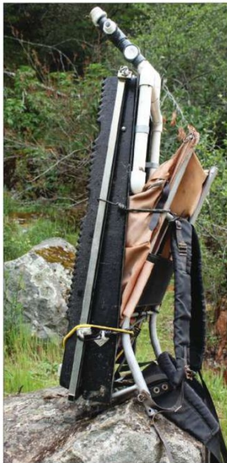
Plastic power sluices are lightweight and can be attached to a backpack with bungees for transporting.
