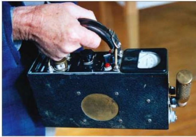
This Geiger counter is typical of those used by prospectors during the post-World War II uranium rush in the Uravan Mineral Belt of Colorado and Utah.
