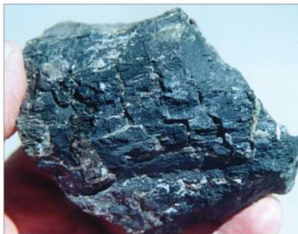
This high-grade specimen of pitchblende (uraninite), an oxide ore of uranium that is found in some pegmatites, has an easily detectable, high level of radioactivity.
