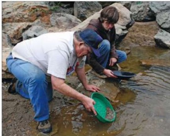
Before moving in your sluice unit, it is prudent to check first with your gold pan and find a good-paying location.
