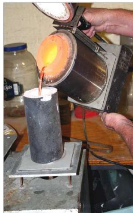
While the molten silver is poured into the hot investment mold, the vacuum pulls air out and silver in.
