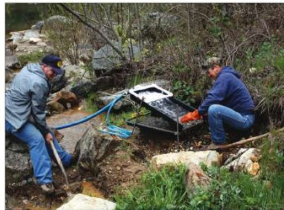
Steve de Caccia and Robert Jordan use a two-part molded plastic power sluice held together by a metal frame with adjustable legs.
