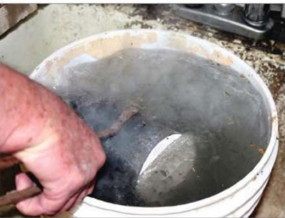
To retrieve the cast silver object, the investment is immersed in water, which breaks it down and releases the object.
