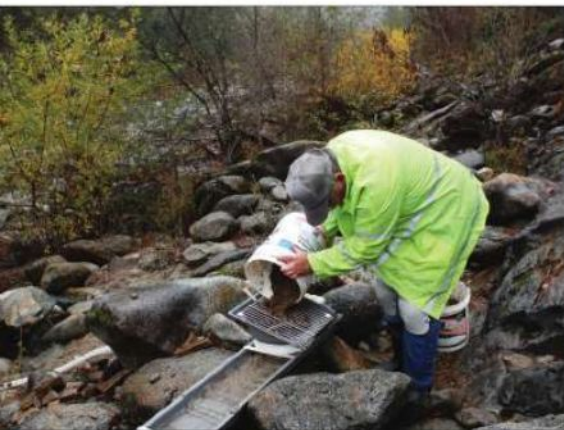
Dirt from on top of bedrock is screened through a grizzly. Undersize material goes into the unit and oversize goes into the tailings.
