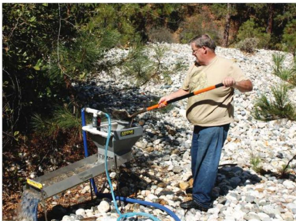
A power sluice does not have to sit in the water to recover gold, but is often set up high above the waterline.
