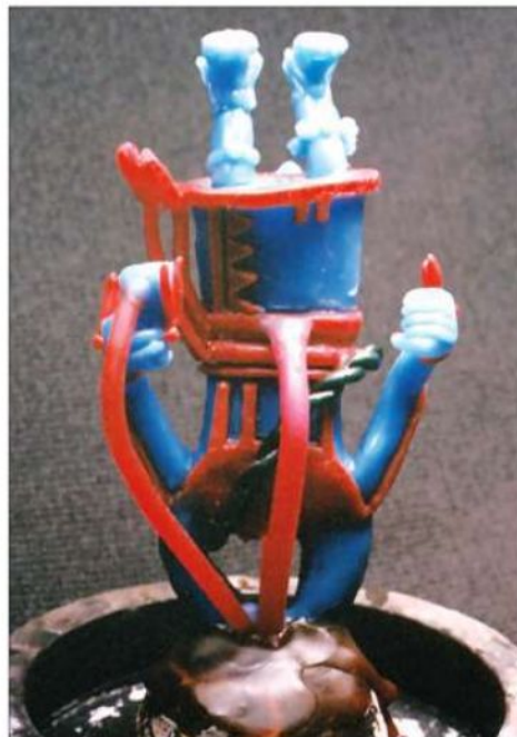
This wax model has sprues attached and is ready to go into the flask for investment.
