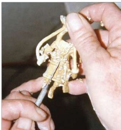
The residual investment is removed from the small and narrow areas with a dental pick.
