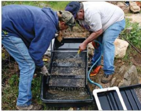
As a lift-out plastic riffle section is washed with a sprayer, the concentrates and gold are caught in a plastic tub.
