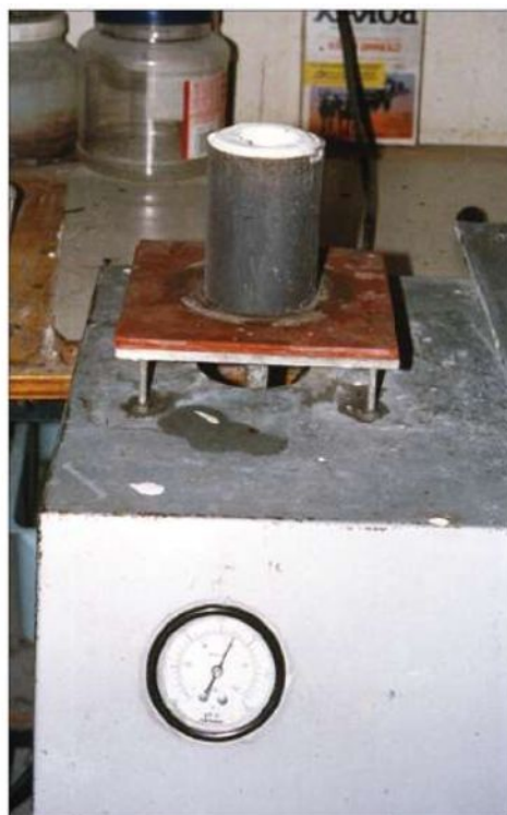
The flask containing the investment mold goes on the vacuum machine, ready for the molten silver.
