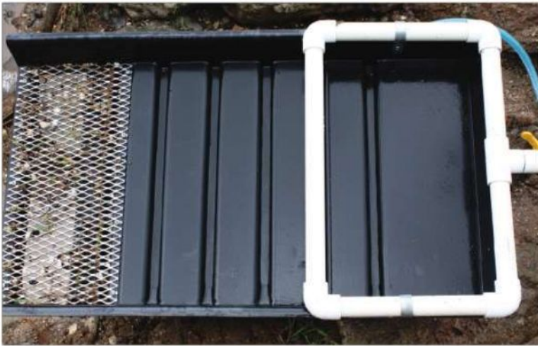
The nugget traps in the upper hopper of this power sluice catch big gold that could otherwise be washed into the tailing pile.
