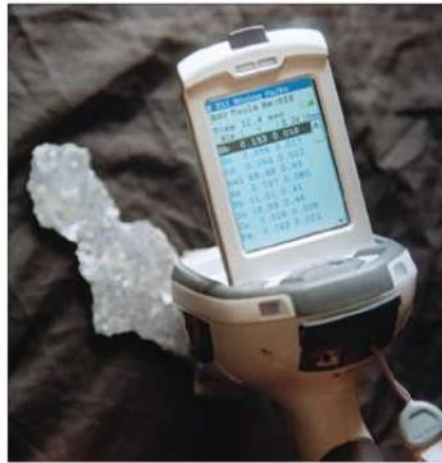
The analysis of a vein center of the famed "amethyst ore" from Creede, Colorado, was performed in 12.4 seconds and showed high values of lead and zinc.
