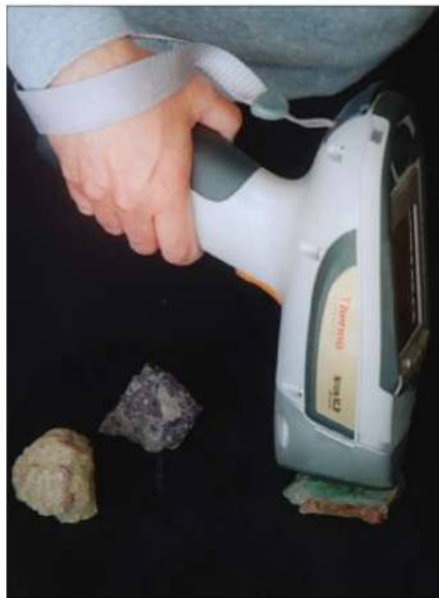
When identifying mineral samples, placing the X-ray window directly against the sample produces the most accurate readings and minimizes X-ray backscatter.
