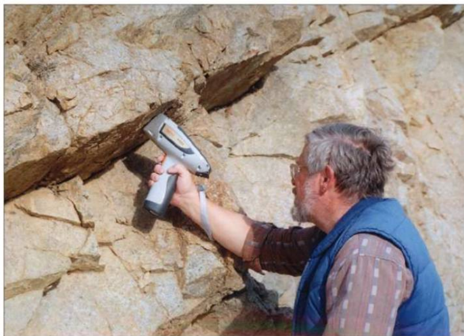
The ability of portable XRF analyzers to obtain accurate, real-time elemental analyses greatly speeds the processes of field mineral exploration and prospecting.
