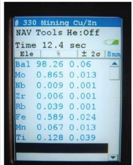
The real-time results of XRF analysis of Climax mine molybdenite ore show lesser amounts of elements so numerous they scroll off the bottom of the screen.
