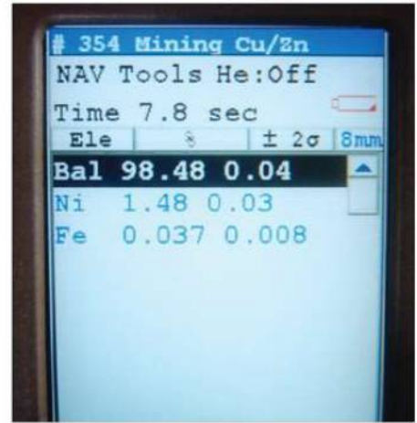
The real-time results of XRF analysis of Australian chryso-prase show a "balance" (silicon and oxygen) content of 98.48 percent, and lesser amounts of nickel and iron.
