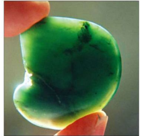
Nephrite and jadeite are chemically and physically similar. Their extraordinary toughness is due to their microscopic textures.
