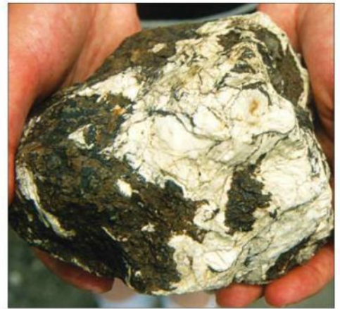
This specimen of high-grade ore from the Smuggler mine contains about 200 troy ounces of silver per ton.
