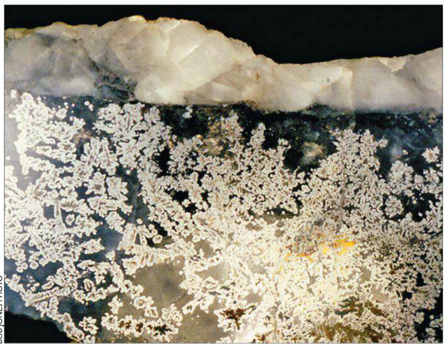
Fragments of diabase rock are held together by sheet silver and cobalt sulfide in this Gioux mine specimen.
