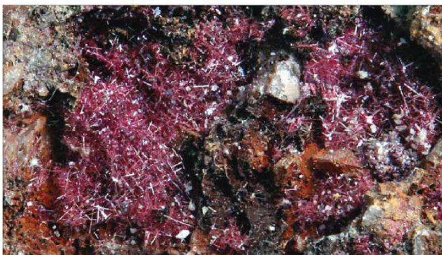
This tangled mass of bright red needles is typical of the copper oxide cuprite, variety chalcotrichite, also called "plush copper". The specimen hails from the Gwennap mines in Cornwall.
