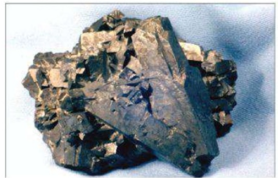
The breakdown of arsenopyrite, an ore of arsenic, releases the element for the formation of Cornwall's rare arsenate minerals.
