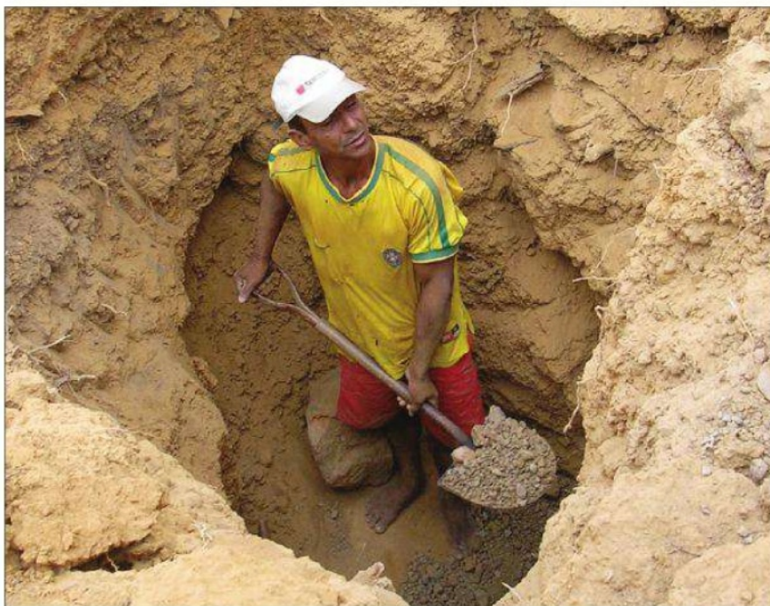
Miners at Ponte do Piauí dig small-diameter holes 6 to 10 feet deep to reach the gem-bearing gravel.
