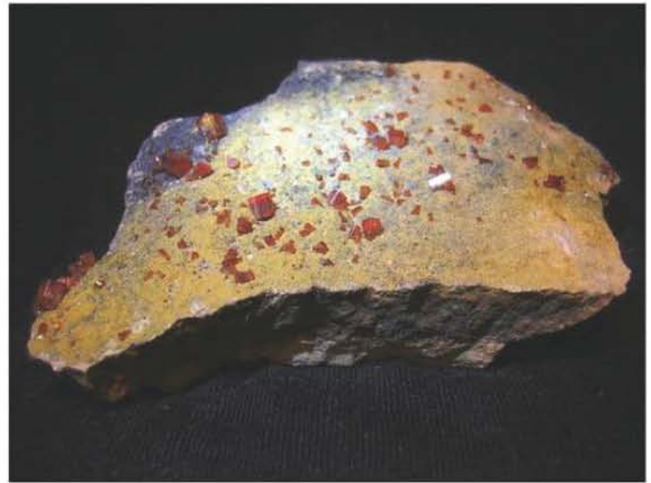
Vanadinite specimens like this one are mined from stratabound carbonate-hosted deposits that rest some 450 feet below ground.
