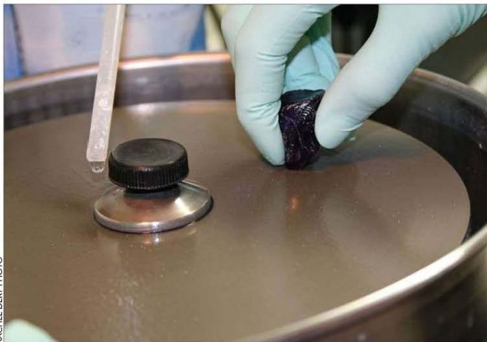
During preforming, I form the rough into the shape I want and take away unwanted material.
