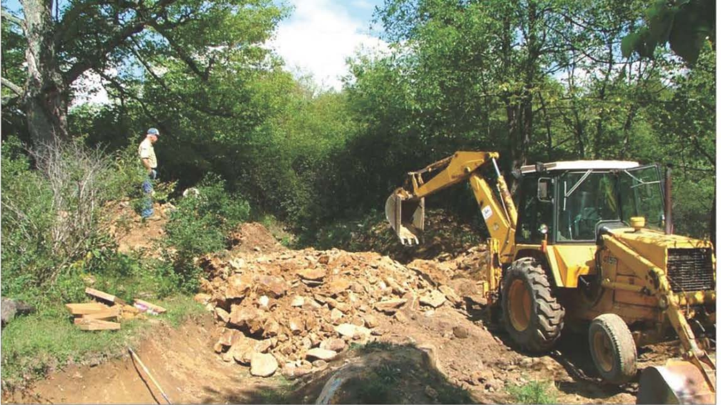
Heavy equipment is useful, but not required, for removing upper soil and rock layers from the mineral-bearing rocks at the Bush Farm collecting area.
