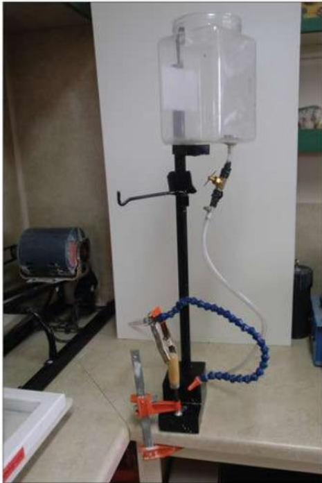
A portable support stand like this one may be used to hold an irrigation supply reservoir.
