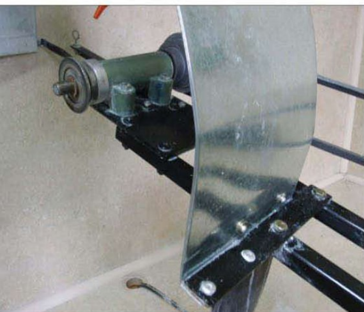
The right side of the fender-style splash shield is attached to the boom arms by means of a stiffening bar.
