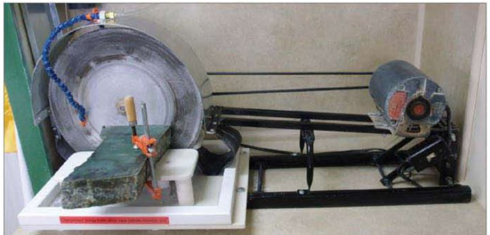
This saw uses a 3/4 horsepower, 1725 rpm, single-phase 60 hz, 115vac motor rather than a 1/2 horsepower motor.
