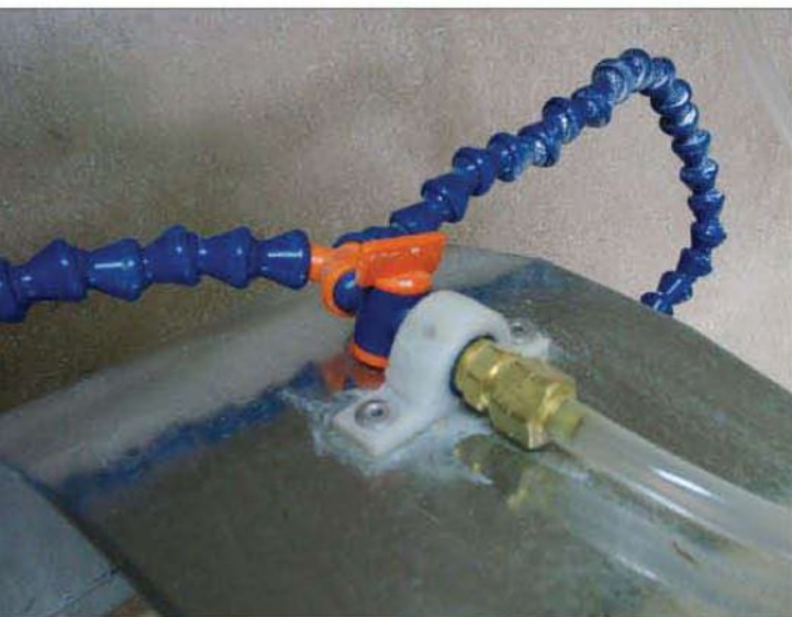
The clear vinyl irrigation supply line connects to a LoLine valve mounted on top of the spray shield, while a Y connector distributes irrigation to both sides of the blade via the adjustable segmented tube.
