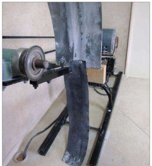
A discarded truck tire inner tube was used to form a flexible spray shield below the rigid metal one.
