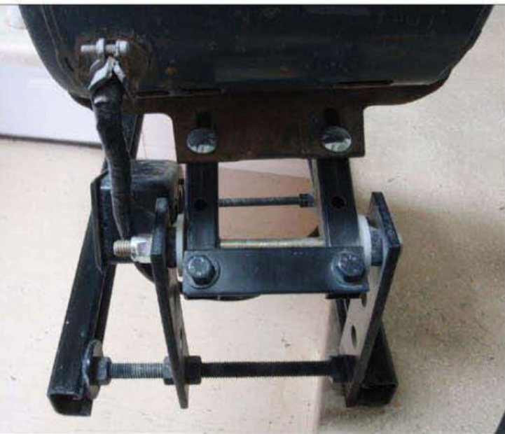
This view rear of the motor shows the necessary bolted cross strap between the boom arms. The nylon washers on the axis bolt ensure smooth pivoting.
