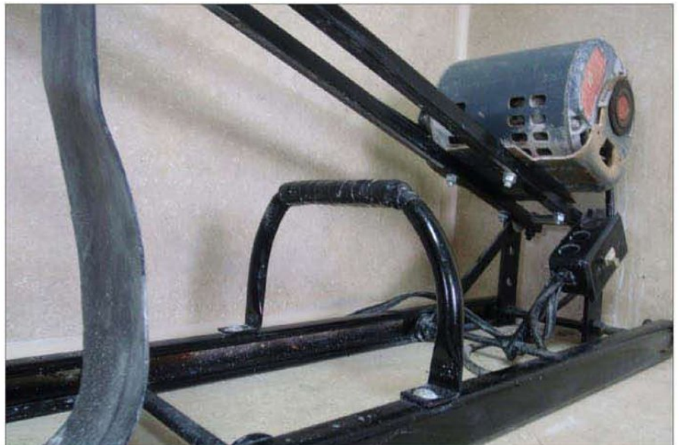
The boom rest prevents the saw blade from penetrating the water collection pan. It was formed from 1/2-inch electrical mechanical tubing (EMT).
