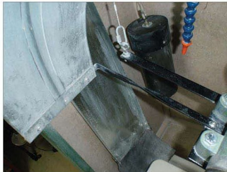
An attachment bar extends from the boom to the bottom end of the light-gauge sheet aluminum splash shield, which is doubled over for strength.
