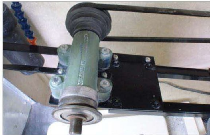
Because the standard ⅝-inch-diameter mandrel mounting holes differed from those on the motor, a steel plate was needed to attach it to the boom arms.
