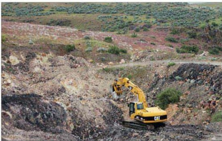
Freeing large thunder eggs from the rhyolite overlay and interburden is nothing less than backbreaking and requires the use of a track excavator and loader backhoe.
