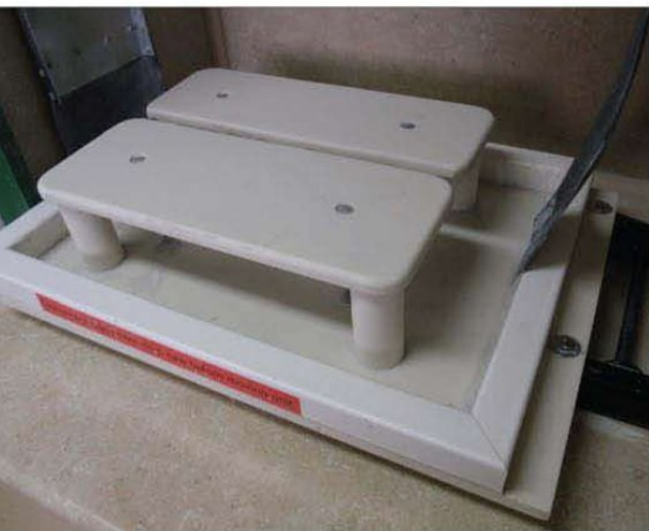
The water collection pan and the stage platforms are made from ½-inch synthetic countertop sheet. The stages are elevated on ½-inch schedule 40 PVC pipe.
