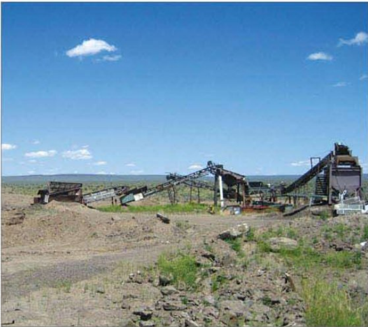
These old belt “picking conveyors”, which will move several tons of rock per hour, are still in use at the Dust Devil mine today.
