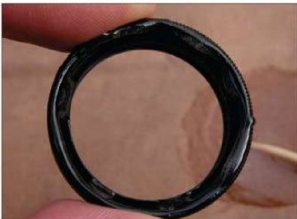
Carefully place epoxy adhesive inside the shoulder of the filter. This will not take much adhesive.
