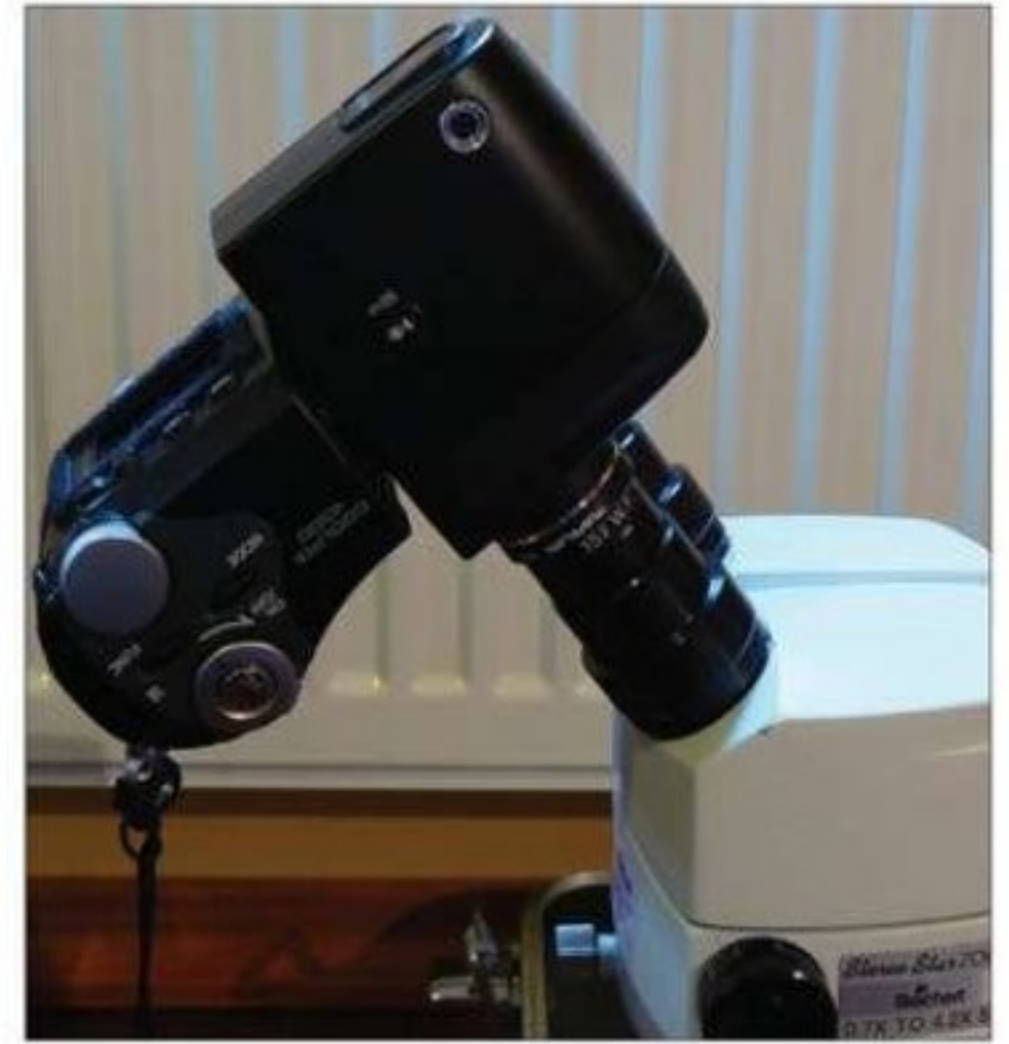
Insert the eyepiece with the camera now attached into the microscope.
