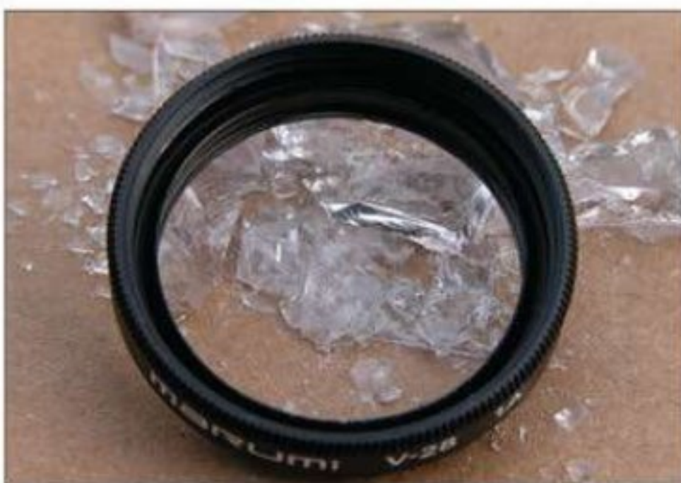
Make sure that all the glass has been removed from the camera filter.
