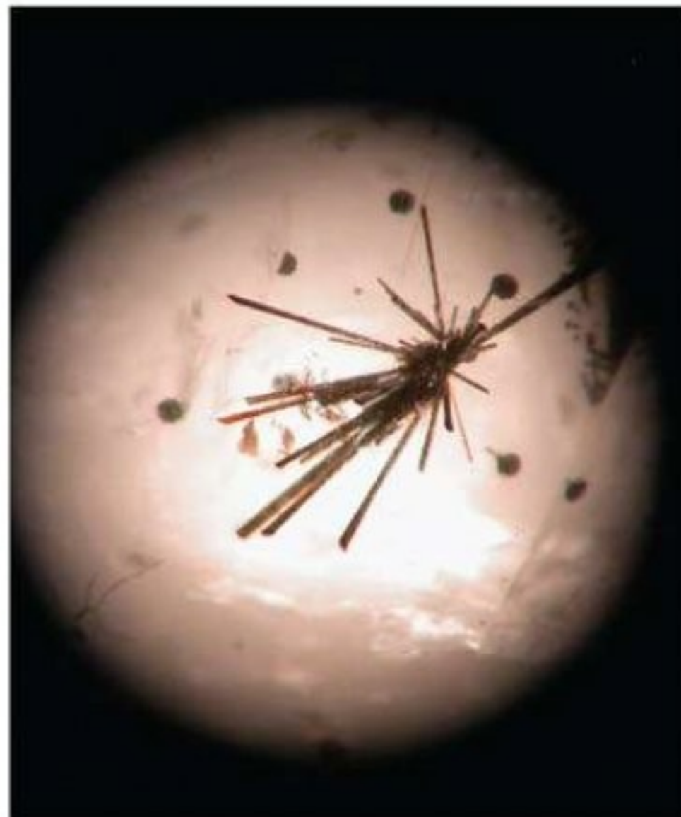
When the camera is first turned on, a large amount of vignetting is seen. Zooming the lens in will eliminate the vignetting.
