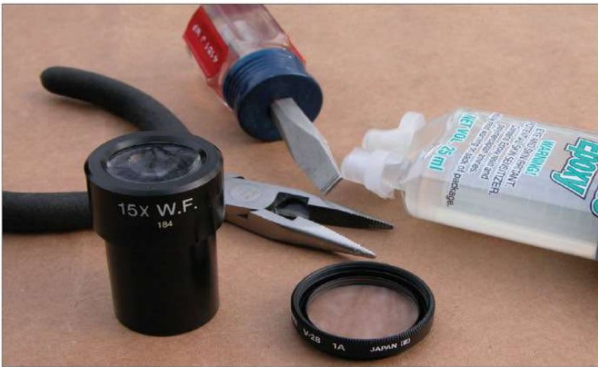
Create the camera adaptor by securing a 28 mm camera filter to the microscope's eyepiece with epoxy.
