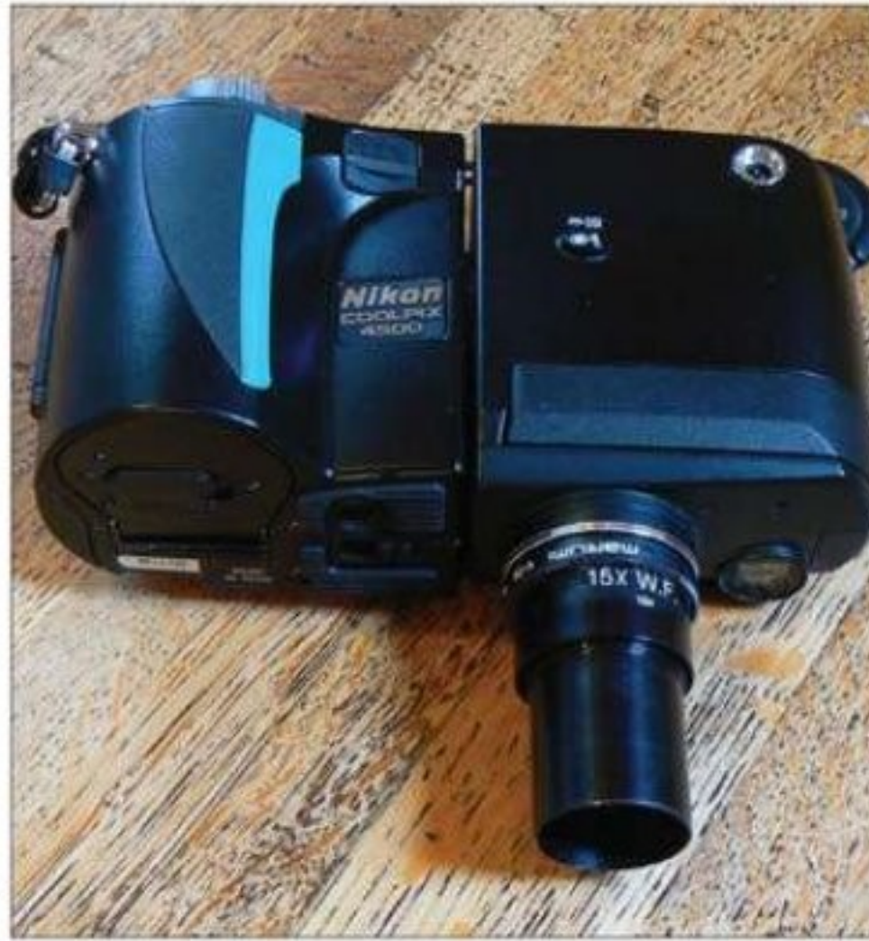
Thread the eyepiece and filter assembly onto the camera and set the camera to macro mode.
