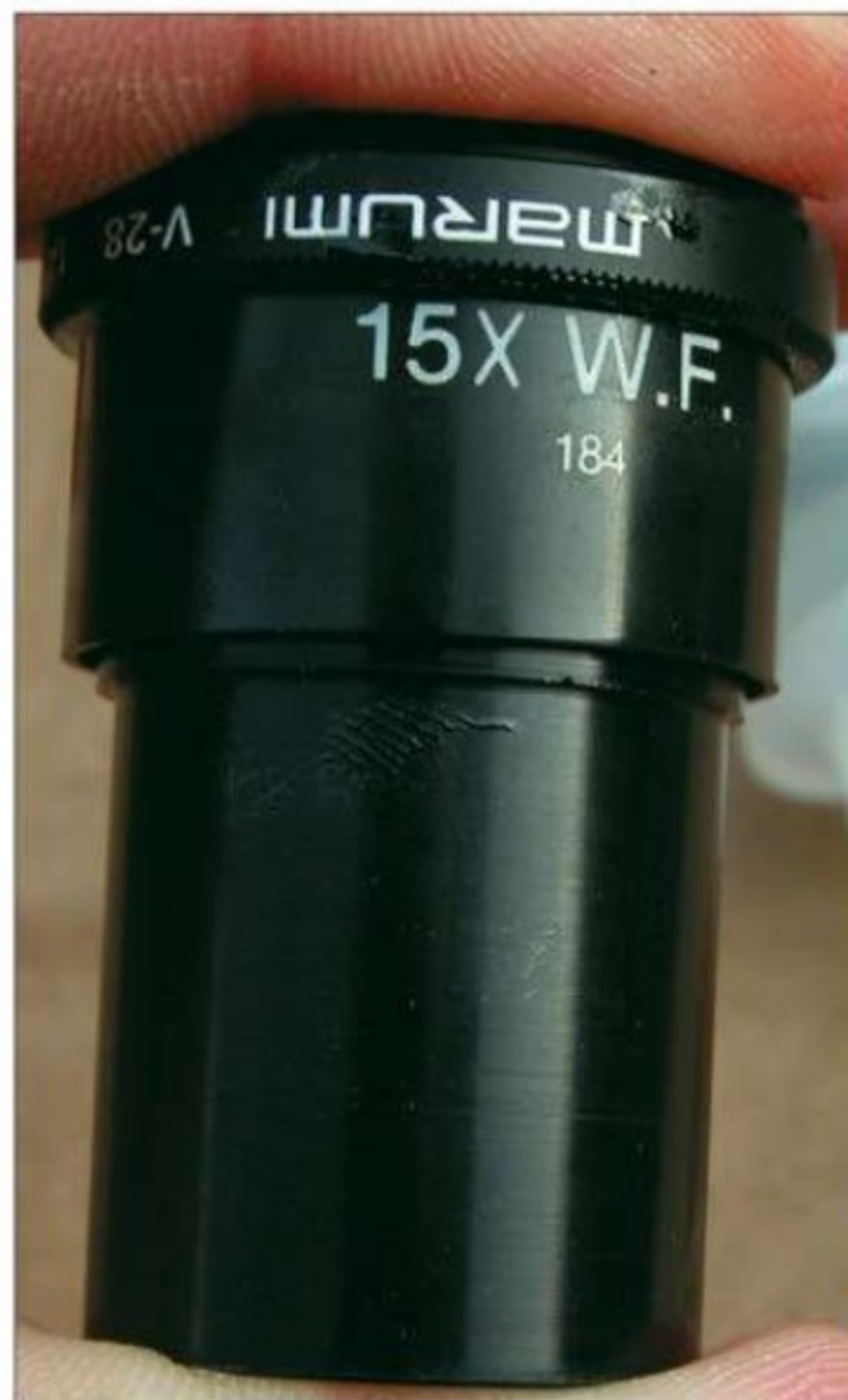
Hold the filter with epoxy in place for the time recommended by the epoxy manufacturer.
