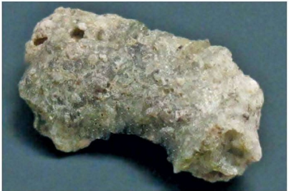
Trinitite is sand that was fused into a crust by the intense heat created by the detonation of a plutonium device.
