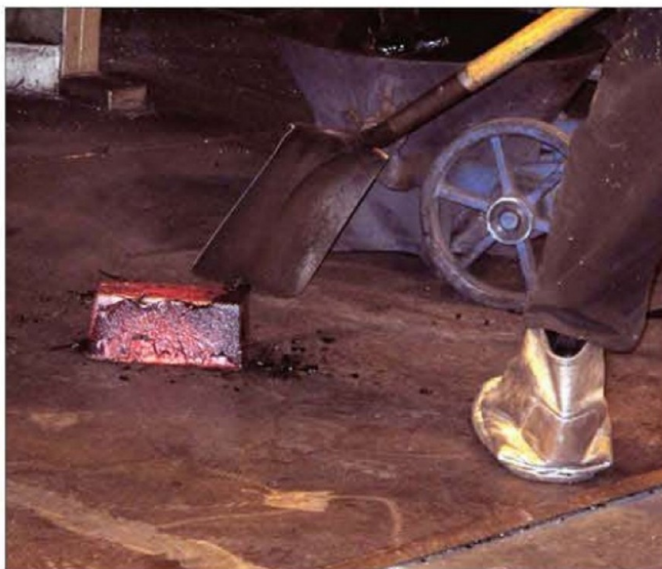
Once the gold is poured, the red-hot gold brick is dumped out onto the steel floor.
