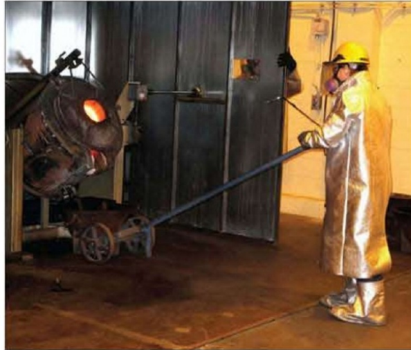
Positioning the mold to receive the molten gold and the slag will flow onto the cone under the mold is very important.
