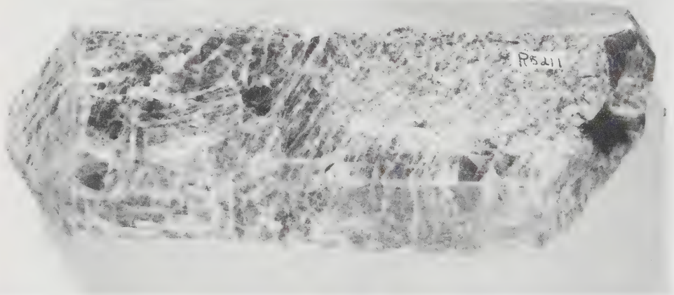
FIGURE 114. A typical Renfrew, Ontario apatite crystal measuring 6 inches long and about 2 inches in diameter; color dark olive green. Although the hexagonal cross-section is apparent in the photograph, none of the crystal faces are very sharp and the "fused" edges so commonly observed in the Renfrew apatites are present. The darker areas to the left are clear and from such places it is possible to cut small faceted gems. Courtesy Smithsonian Institution.
