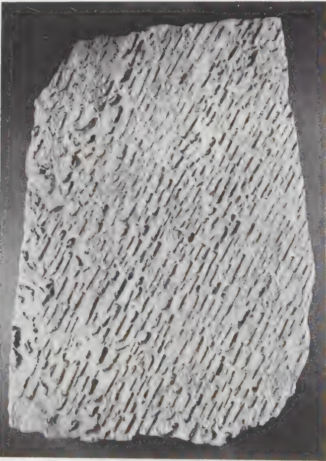
FIGURE 148. Polished slab of graphic granite from Hybla, Ontario, measuring 15 inches by 11 inches. The rock consists entirely of flesh-pink feldspar penetrated by angular inclusions of smoky quartz. Courtesy Smithsonian Institution.
