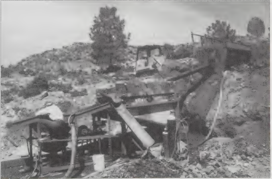
FIGURE 7. Washing rig recovering benitoite and other minerals from the alluvial material below the deposit outcrop, San Benito Co., CA. Courtesy Michael Gray.
