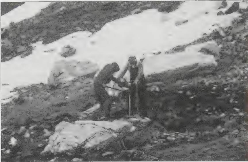
FIGURE 40. A diamond core-drill being used to test a talus block of nephrite on a mountainside in the Dease Lake area, British Columbia. Courtesy S. F. Leaming, Summerland, B.C.
