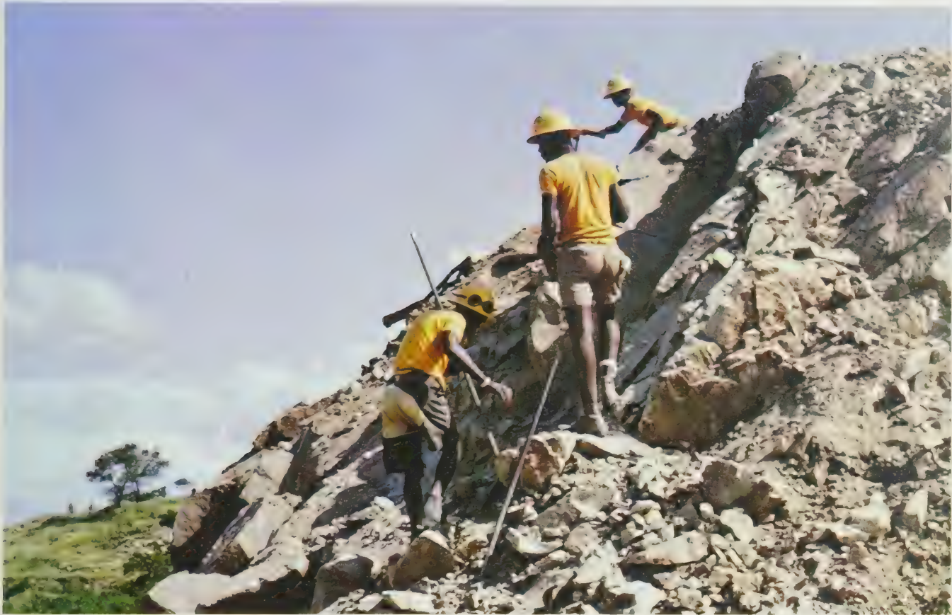
34 Miners break up the loose rocks of an emerald deposit with crowbars.
