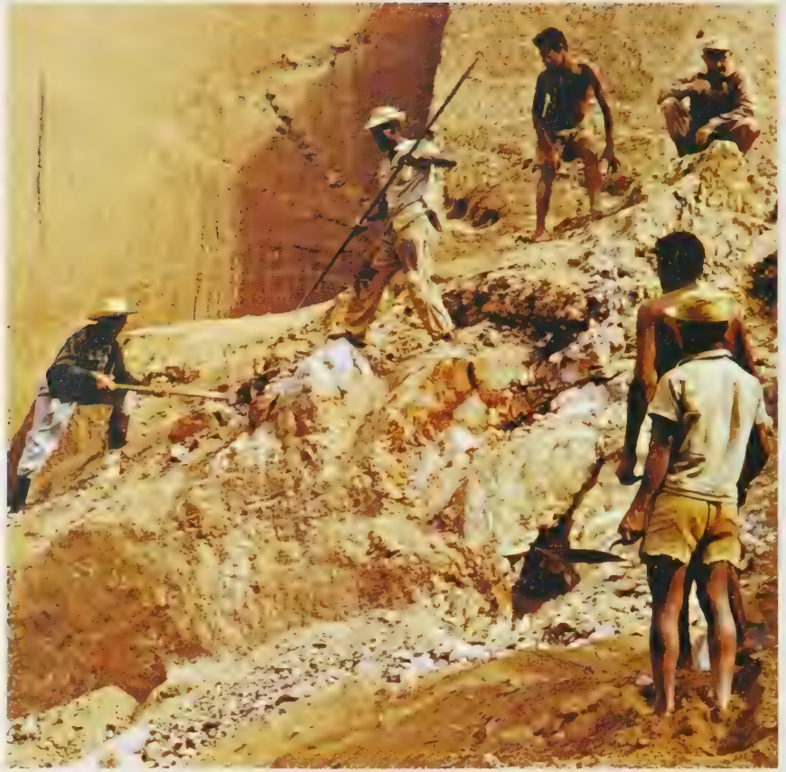
31 In the quarrylike open-cast mine of a primary deposit of aquamarine near Pedra Azul in Minas Gerais, Brazil, miners are in the process of breaking up the matrix (pegmatite).
