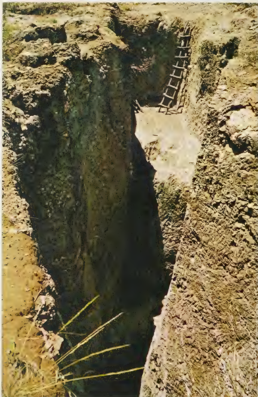
41 Steplike mine producing garnet and corundum from secondary detrital sediments of the Umba River in Tanzania.
