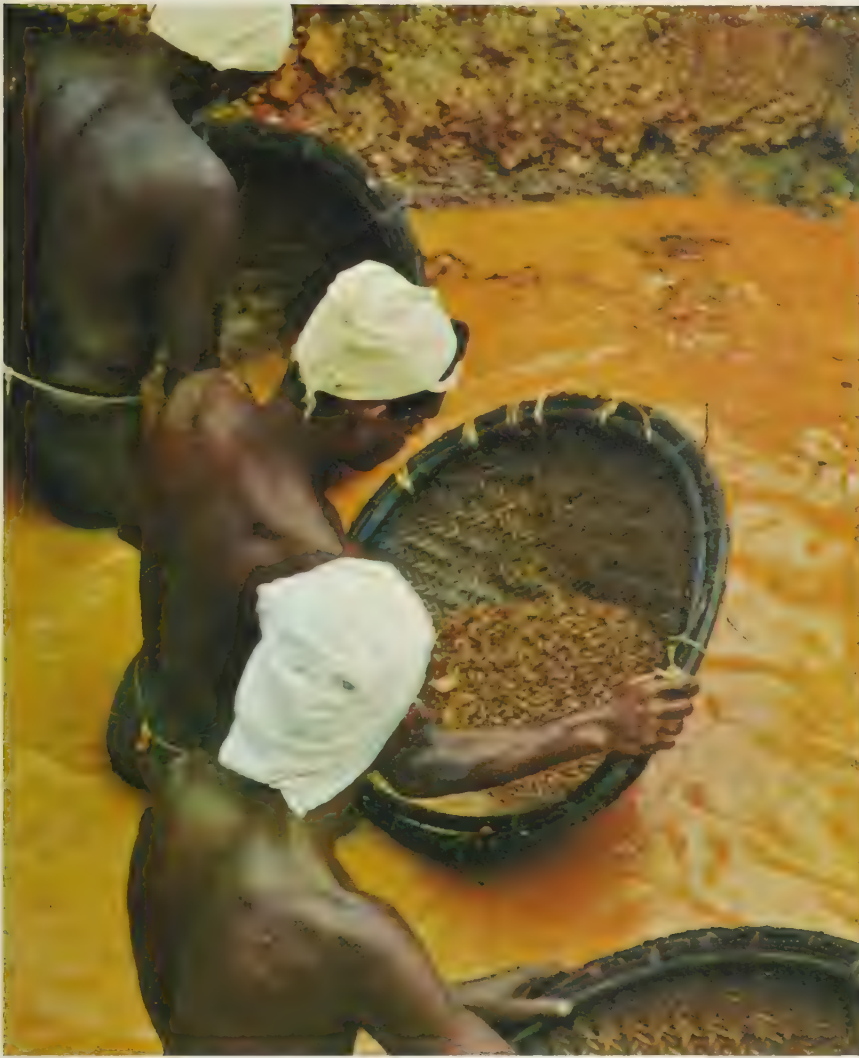
39 The puddlers fill their conically woven baskets at the pile of illam and carry them to the wash pool. Here they stand up to their waists in the muddy water and rotate their baskets so skillfully that all light and worthless material is floated over the edge of the basket, while the heavy gemstones—chrysoberyl, garnet, corundum, spinel, topaz, tourmaline, zircon, and many others—collect in the deepest part of the basket as so-called “dullam.” The washer fills and washes his basket several times until sufficient dullam has collected in it. Then he places the basket in front of the overseer and the exciting moment has come.
