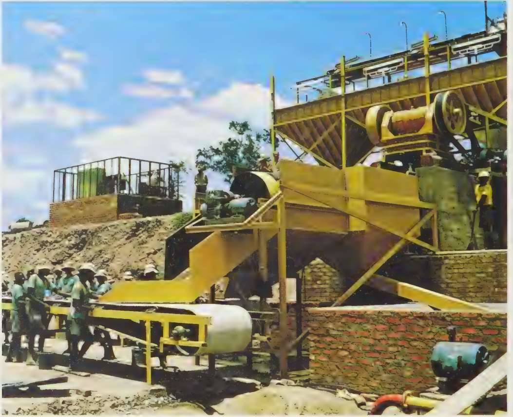
35 At the Somerset emerald mine in the Transvaal the emeralds are loosened from their matrix in huge concentration plants, and, underneath, are picked by hand from the conveyor belt by sharp-eyed workers.
