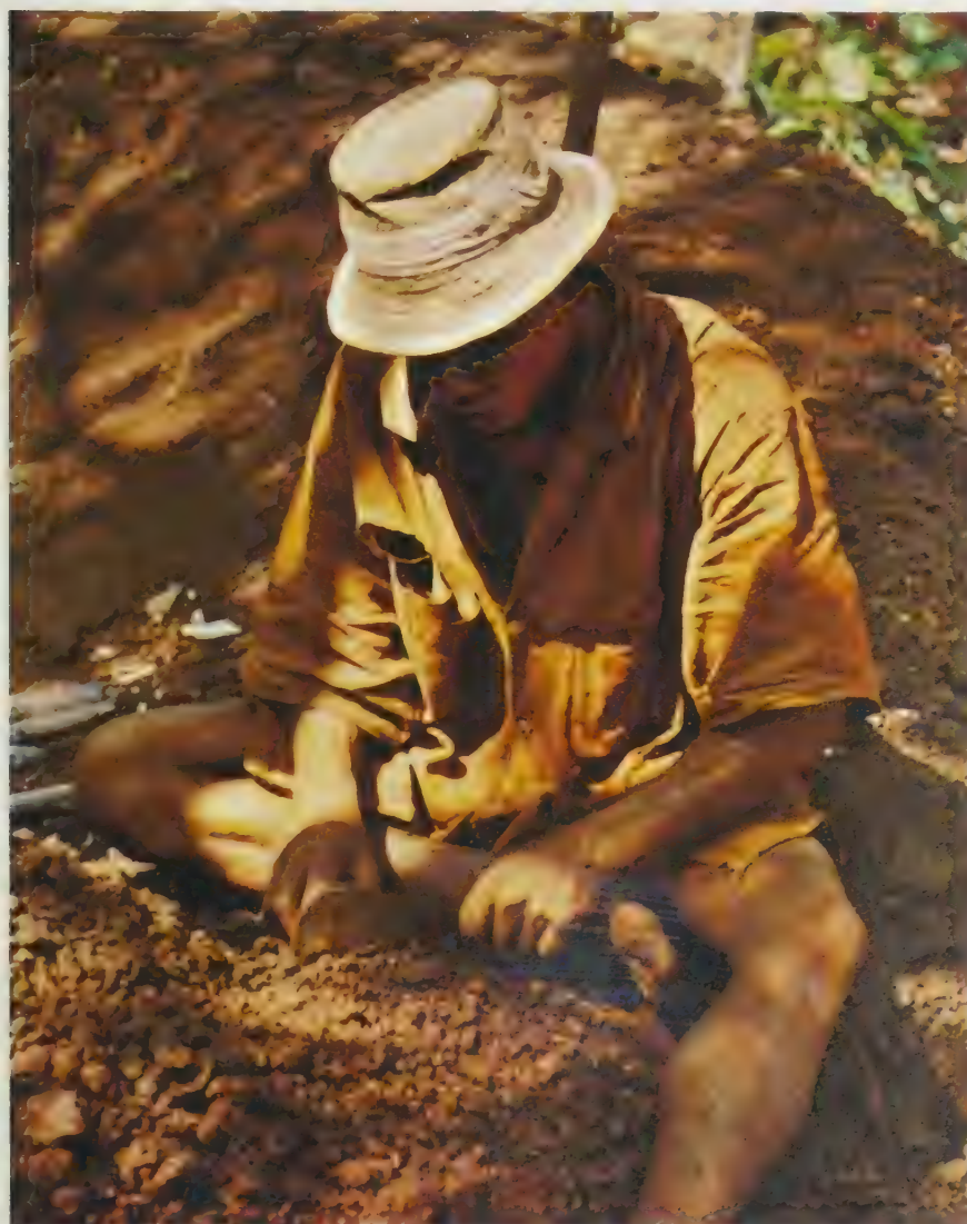
29 The gem-bearing gravels are dumped near the mouth of the pit. From time to time the miner squats down on them and searches through the mine spoil with a scythelike tool. Only where water is available are they washed. A lovely variety of corundum occurring here is the yellow- and blue-, as well as green- and yellow-banded sapphire. As elsewhere, there are varying qualities here, too.
