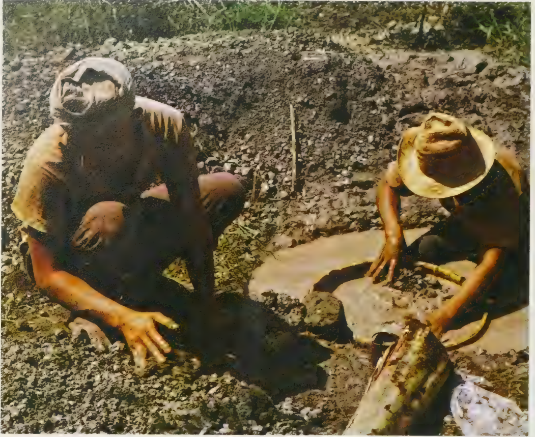
60 Zircon washers buddle the excavated gravel in a small water hole on a zircon field in Cambodia.
