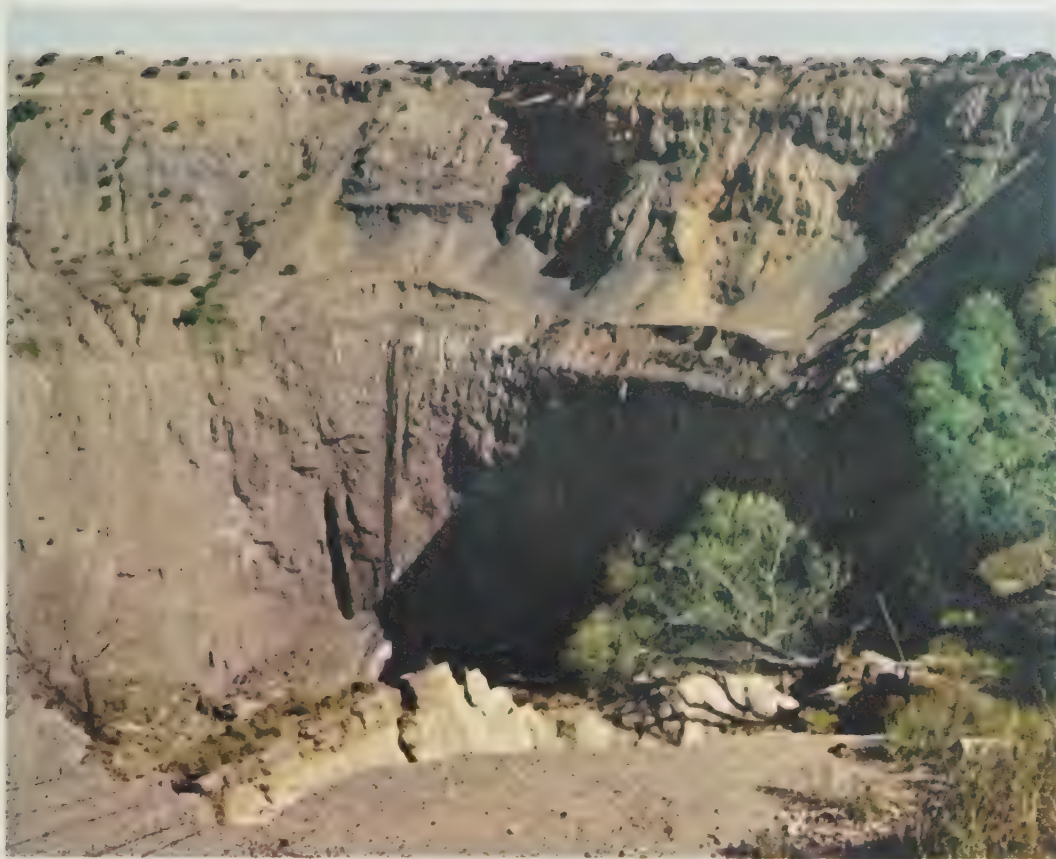
14 Crater of a so-called pipe mine in South Africa, mined by open cast methods.
