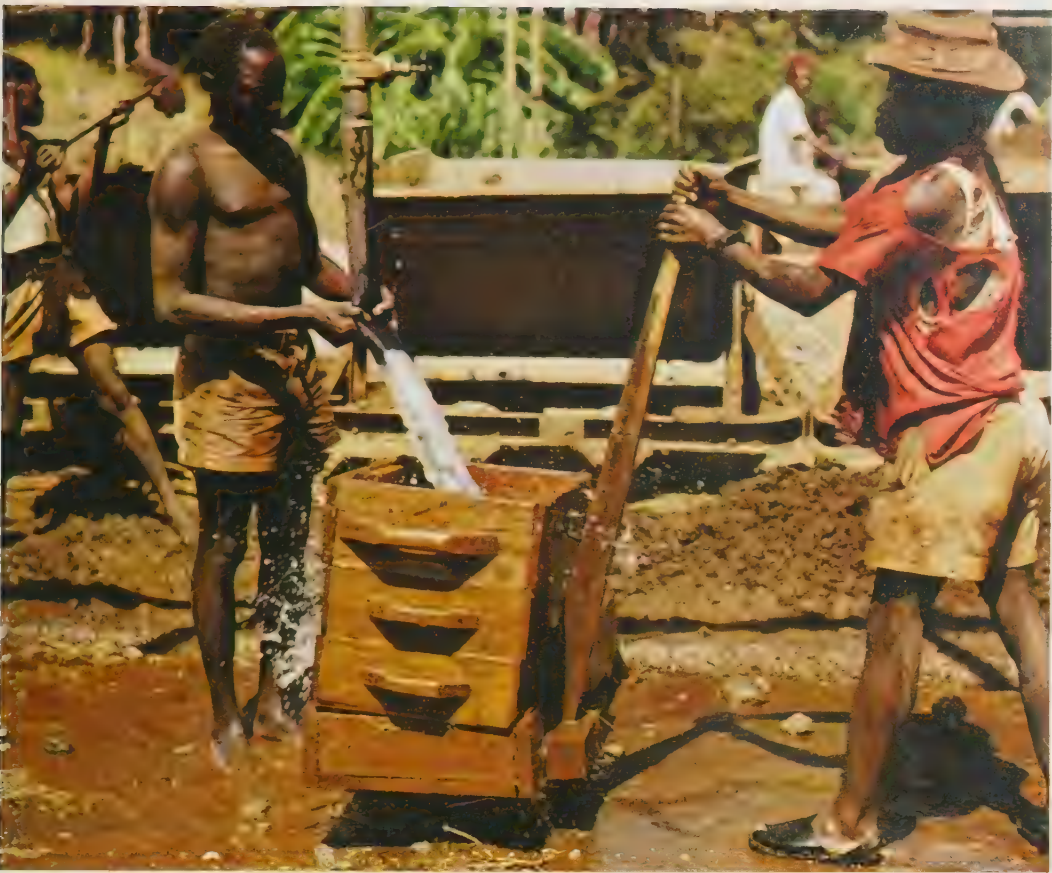
42 Separating jig with sieve boxes for recovery of garnets and corundum from the Umba River in Tanzania.
