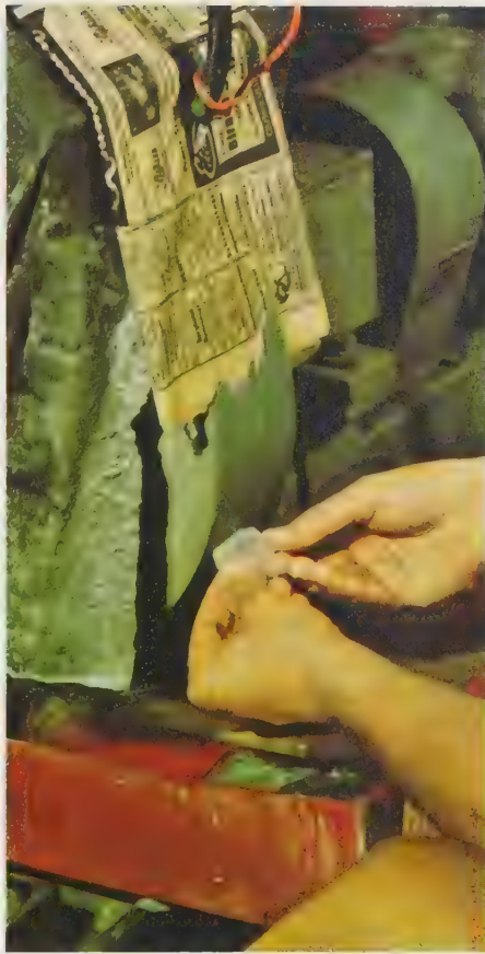
11 On the grinding wheel the gems are ground into a rough, preliminary shape.
