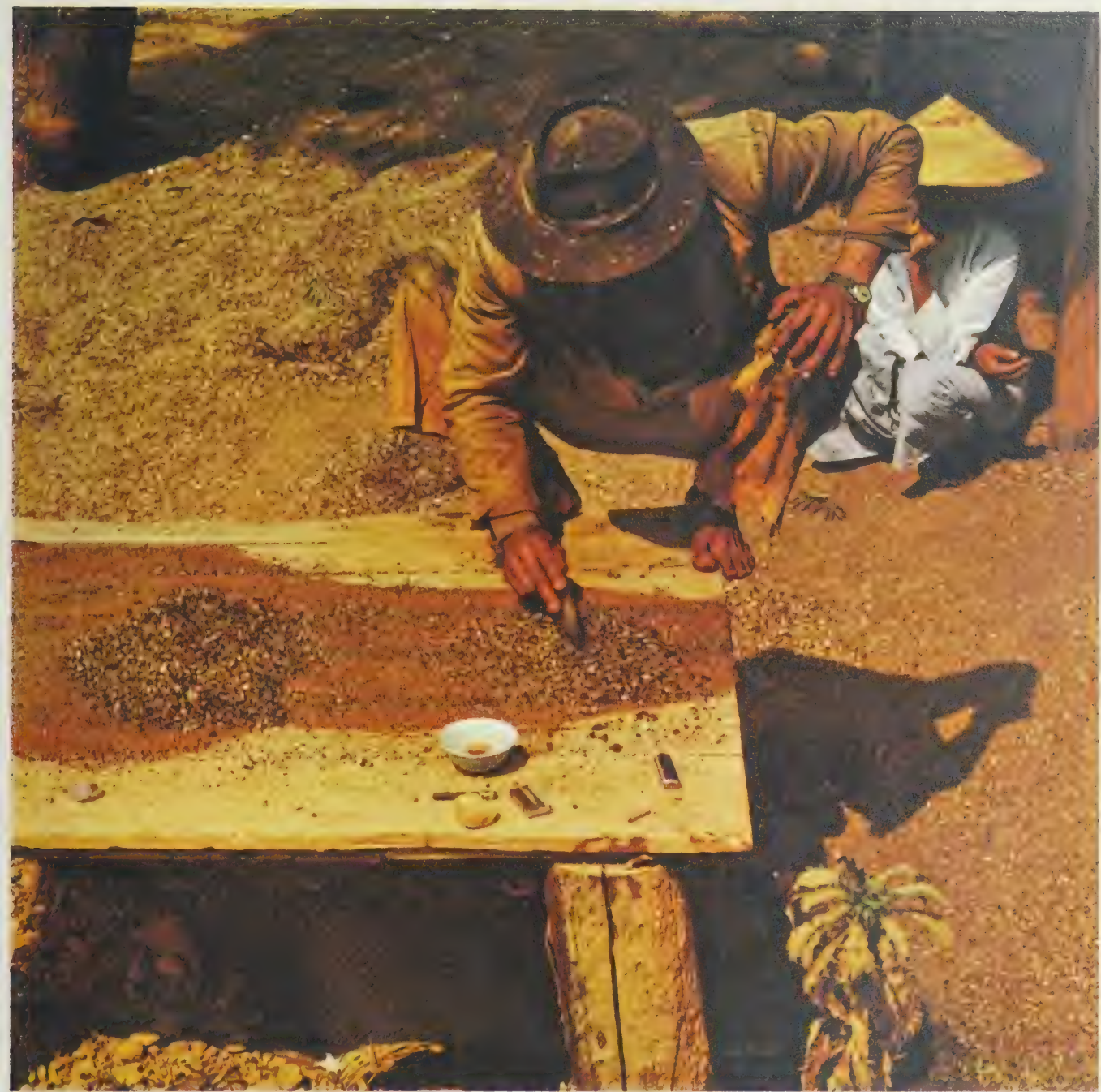
25 The concentrate is scooped out by hand, for spreading out on the sorting table. Squatting at the sorting table, the sorter, with scarcely contained excitement, takes out from a multitude of worthless pebbles a few tiny red sparkling grains and puts them carefully away in a silk purse. As reward for his tedious work the earth has given him a few small rubies. On the primitive cutting benches, whose laps are foot-driven, the rubies receive their richly faceted cut form.
