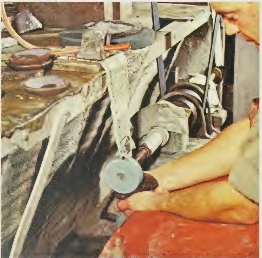
77 The cutter of bowls holds the bowl between his knees against the cutting wheel to obtain surer and steadier control.
