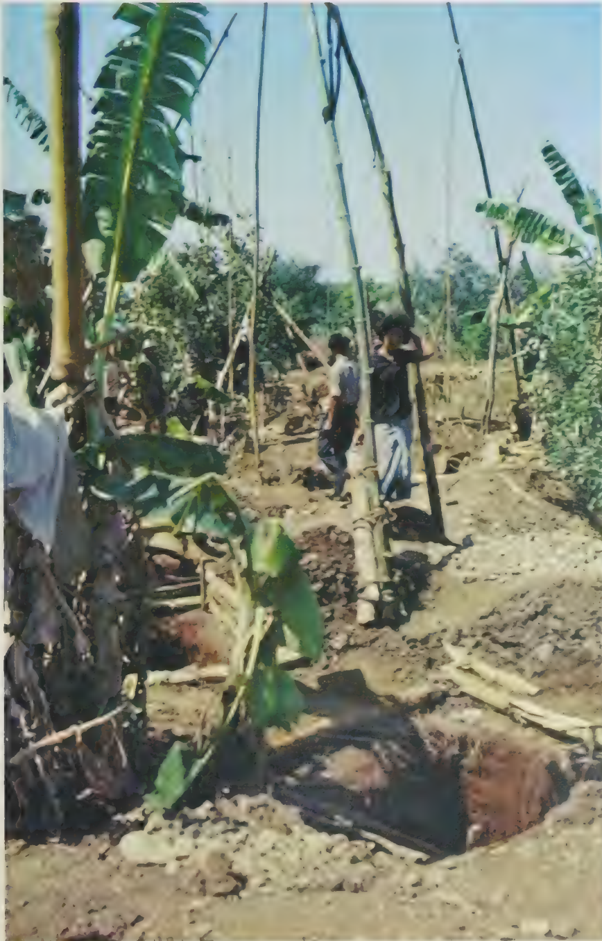
28 In the very prolific sapphire deposits near Kanburi and Bang-Kha-Cha in Thailand and Pailin in Cambodia, which were discovered between the midnineteenth and twentieth centuries by migrant Burmese, the extraction methods introduced by them have scarcely changed. Often the fields of diggings lie in abandoned banana or rubber plantations. The deep, narrow excavations are usually small family concerns. In many places they are connected up together by crawling tunnels. At depth a man digs up the riches of the earth and heaps the spoil into plaited bamboo baskets. At the top a woman looks after the bamboo hoists, to which the baskets are attached when full.
