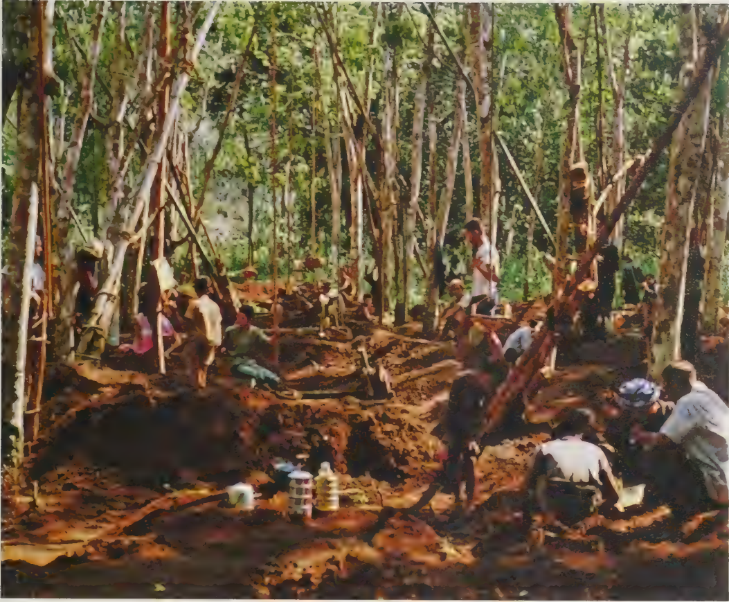
61 Former rubber plantation with innumerable mounds thrown up from small zircon mines. Some of them are being excavated and the spoil is being brought up in baskets on a bamboo hoist, while at the edge of other holes the dug soil is being sifted.
