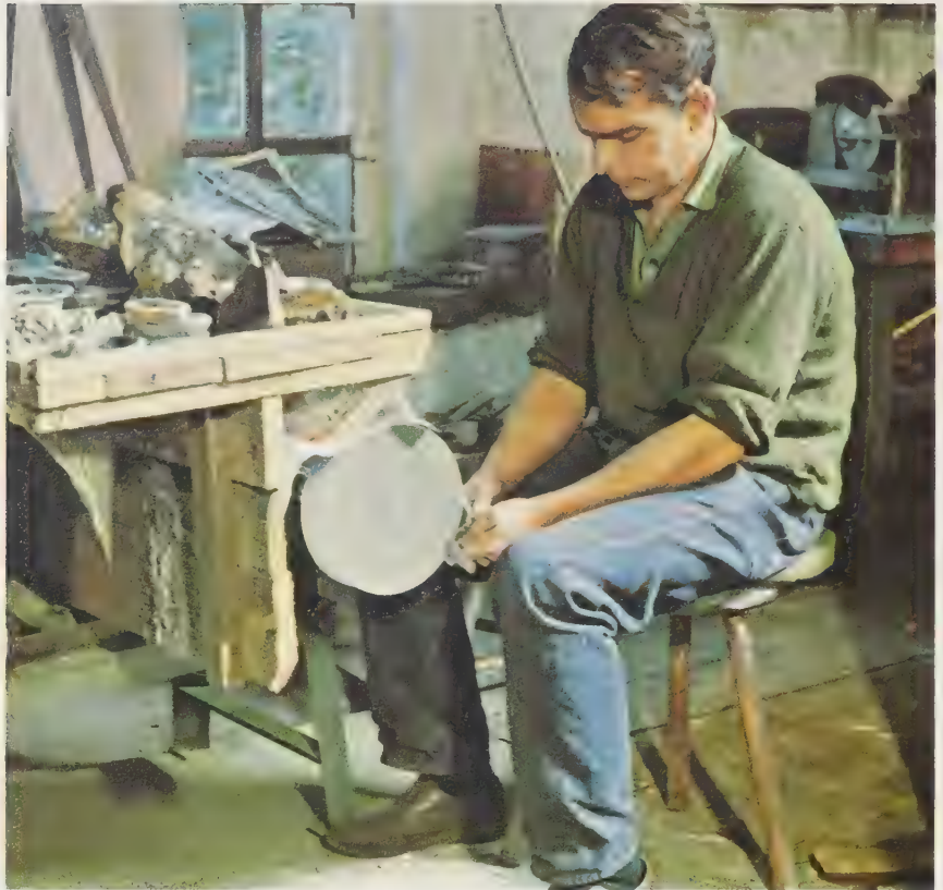
76 Smaller pieces of agate receive the rough shape of their final form on the coarse grinding wheel.
