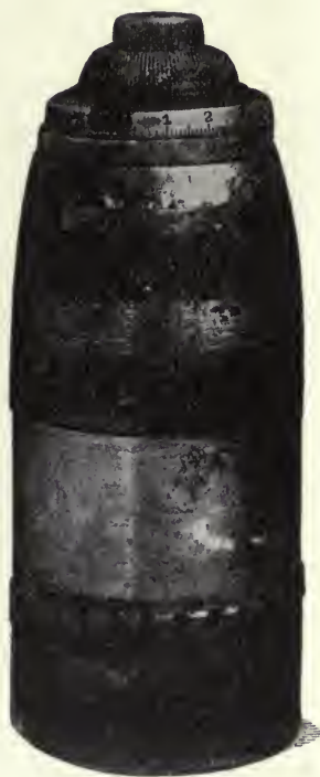
Boer 9 lb. Shrapnel, \frac{1}{4} Actual Size, showing Time Fuse.
