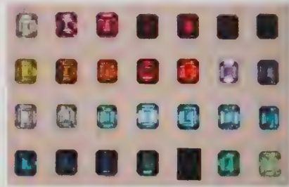
TOP: Synthetic spinel boule ABOVE: Colours produced by the flame fusion process
