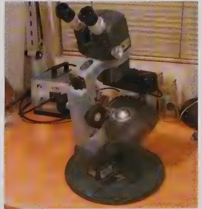
ABOVE: A binocular microscope with dark-field illumination, overhead lighting and an independent fiber optic light source is the instrument of choice for detailed forensic work and other more difficult cases
