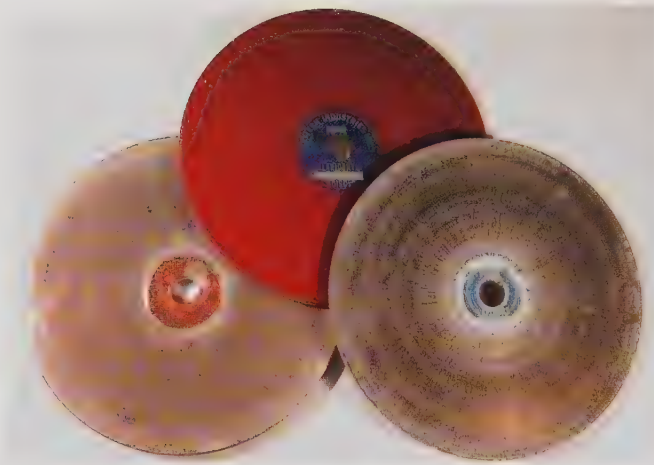
LEFT: Basic laps (from left to right): sintered diamond cutting lap; colored phenolic polishing lap; tin lap with radiating grooves
