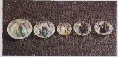
ABOVE: Dispersion in the following gems (from left to right): synthetic rutile, strontium titanate, moissanite, cubic zirconia, diamond
