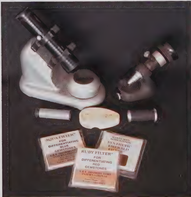
LEFT: Spectroscopes (LEFT), dichroscopes (RIGHT), Chelsea color filter (CENTRE), and color filters (BOTTOM)
