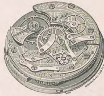
No. 90 —Gilt, Fifth Second Chronograph, with Start, Stop and Fly-Back working from the Pendant, Nine Jewels, Cur Expansion Balance, fitting all regular 18-size Open-Face Cases, and warranted in every respect, Plain or Fancy Dial.
