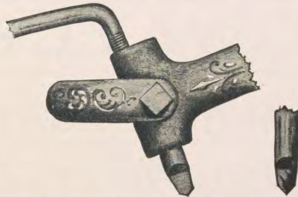
Fig. 1 Fig. 2 "From a hair line to a broad, bright cut, in a second"—just as by hand. Fig. 1 shows angular adjustment of graver on an Eaton-Engle that gives those elegant, bright cuts, that have made our machine famous. Fig. 2 shows vertical position in which graver is always held on all other styles of machines made previous to ours. Is it any wonder they only did "scratch work"?
