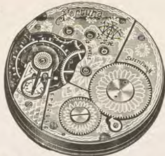
No. 125. "FORTUNA." 16 Size, 12 Jewels. Solid nickel top plate handsomely damaskeened in gold, micrometer regulator, cut expansion balance, safety pinion, screw bankings, straight line lever escapement, hardened and tempered breguet hairspring, quick train, exposed winding wheels, dust band, handsome white enamel dial with depressed second and center and with red marginal figures. Hunting lever set. Open-face pendant set. Price, $9.50.
