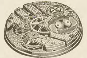
No. 300. "FORTUNA." 6 Size, 7 Jewels. Nickel damaskeened, cut expansion balance, safety pinion, screw bankings, straight line lever escapement, hardened and tempered breguet hairspring, quick train, exposed winding wheels, handsome white enamel dial with depressed second and red marginal figures. Stem wind and lever set. Price, $5.00.
