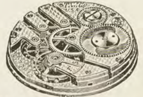
No. 300. "FORTUNA." 6 Size, 7 Jewels. Nickel damaskeened, cut expansion balance, safety pinion, screw bankings, straight line lever escapement, hardened and tempered breguet hairspring, quick train, exposed winding second wheels, handsome white enamel dial with depressed second and red marginal figures. Stem wind and lever set. Price, $5.00.
