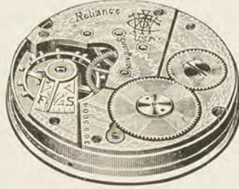
No. 200. "RELIANCE." 16 Size, 7 Jewels. Nickel damaskeened, cut expansion balance, safety pinion, screw bankings, straight line lever escapement, hardened and tempered breguet hairspring, quick train, exposed winding wheels, dust band, handsome white enamel dial with depressed seconds. Hunting lever set. Price, $6.00.
