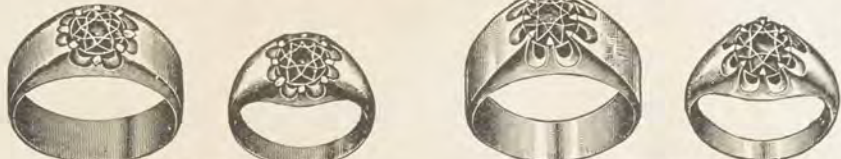
These two cuts show Flat and Round Belcher Rings as received, with claws badly worn off and too low to permit resetting stones again.
