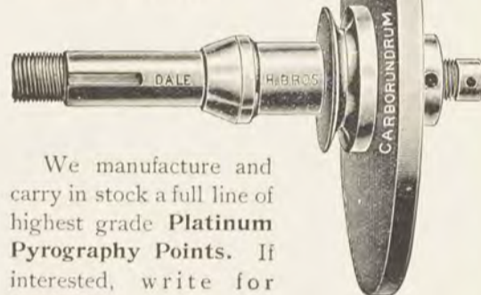
CARBORUNDUM WHEEL AND MOUNT Price, fitted to any standard watchmaker's lathe, $3.50
