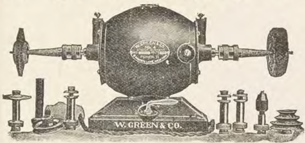
This is our No. 4, 1905 Model Direct-Current Lathe
