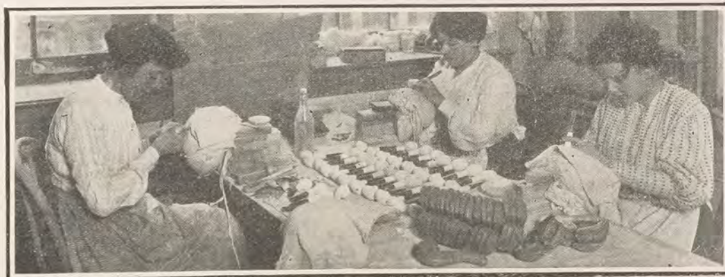
Smoothing off the pipes with shave grass
