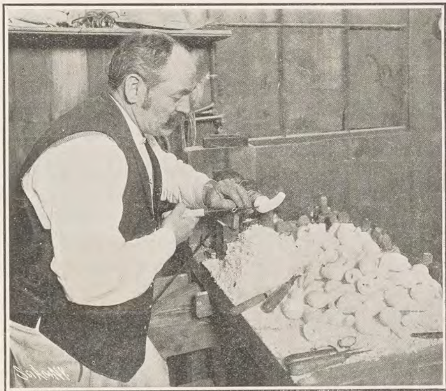
Turning up the bowls and stem shanks
