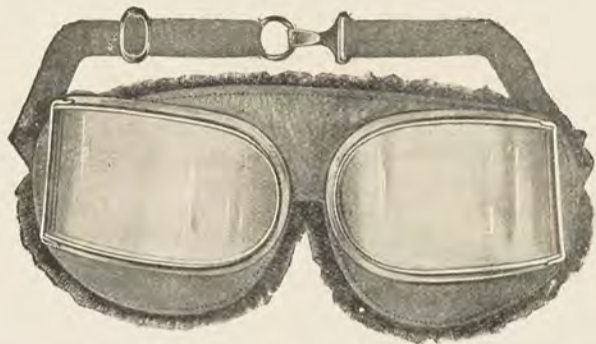
Aluminum frame, extra large bent glass, 1\frac{5}{8} \times 3\frac{1}{4} inches giving unobstructed wide field of vision. Leather mask, lined with green silk, bound with chenille.
