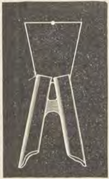
Fig. 44 Home-made form of Hering's Drop Test.
