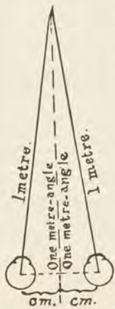
Fig. 4 Shows how 1 m. a. contains as many sine centunes as there are centimeters in half the interocular distance.
