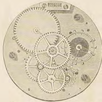
THE TRENTON WATCH MOVEMENT WITH TOP-PLATE REMOVED.
