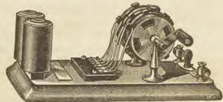
Greaves' Demagnetizer (Patented).
