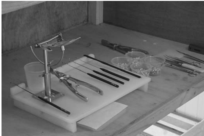
FIGURE 8.11 Specialized tools used by grafting technicians. On the left of the board is the shell stand used to hold the oyster to be operated, with the speculum (used to hold the oyster open) to the right of the stand. A range of different sized nuclei are held in the plastic containers to the right. Other tools are used for cutting and placing the nuclei and mantle tissue within the oysters, and the small board covered with white absorbent paper at the front is used to hold the mantle tissue sections. (Photo: Paul Southgate.)
