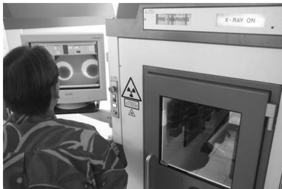
FIGURE 9.18 Black pearls being X-rayed to determine nacre thickness as part of French Polynesian government measures to maintain quality of exported pearls. The operator views X-ray images of the pearls (in the X-ray machine on the right) which clearly show pearl nuclei and nacre thickness.
