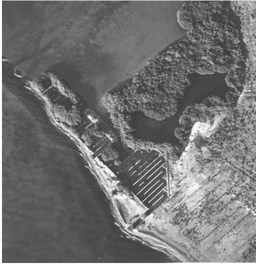
FIGURE 9.23 Aerial view of the remains of the Compañía Criadora de Concha y Perla de Baja California Sur, S.A. (CCCP) at Bahía San Gabriel, Espiritu Santo Island near La Paz, Baja California Sur. The nursery culture channels were constructed within an artificial lagoon and used to house wire cages containing Pinctada mazatlanica .
