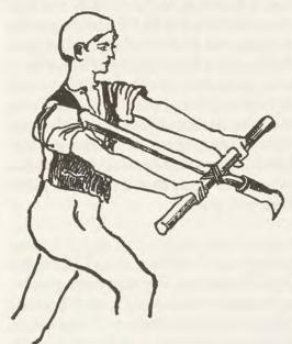
You make your silver plate red hot & place it on one of the iron plates you used for casting it on; fastening it on tightly with certain iron tools used for nailing or fastening, then setting the handle of the scraper to your shoulder with your two hands to the two handles that you fastened to it, so that it comes to be in the form of a cross, you pare off the surface of your silver plate with very firm pressure till it is thoroughly clean.
