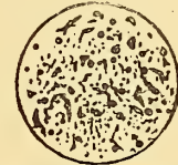
FIG. 2.—Spherical and irregular cavities in artificial ruby as seen at one time, evidently from the lower part of the crucible (enlarged 25 diameters).
