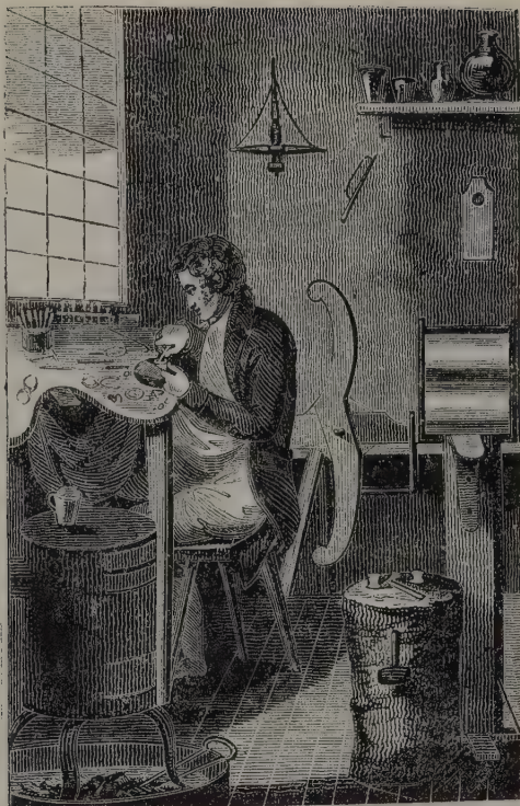
Fig 3.6 A London jewellers' workshop in 1811, showing workboard, drawbench, flatting-mill, stake-block and furnace.
