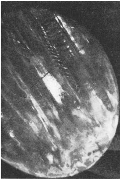
FIG. 1. Synthetic black opal (Gilson, early 1974) showing longitudinal banding, with some "herringbone" structure; note "equigranular" appearance near bottom of photograph. \times 4.5 , reflected light.
