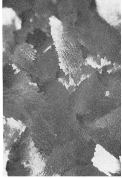
FIG. 8. Synthetic black opal (Gilson, Dec. 1975) showing "lizard skin" effect and crenulate margins. \times 12 , reflected light.
