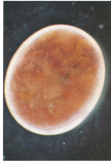
FIG. 6. Synthetic white opal (Gilson, Nov. 1975) showing pinkish-buff matrix colour, pale pink, blue and yellow patches and "dried leaves" effect. \times 4 , transmitted light.
