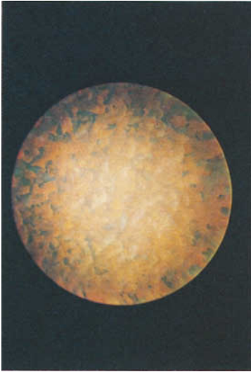
FIG. 3. Synthetic white opal (Gilson, late 1974) showing "equigranular" mosaic. \times 5 , transmitted light.
