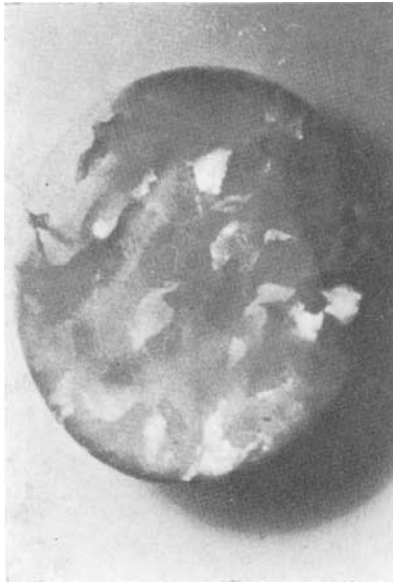
FIG. 9. Synthetic white opal (Gilson, Nov. 1975) immersed in chloroform showing transparency spreading from girdle at top left. \times 5 , reflected light.
