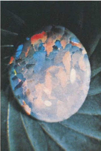
FIG. 13. Synthetic black opal (Gilson, Dec. 1975) showing mosaic with distinctly crenulate boundaries and "lizard skin" effect. \times 4 , reflected light.
