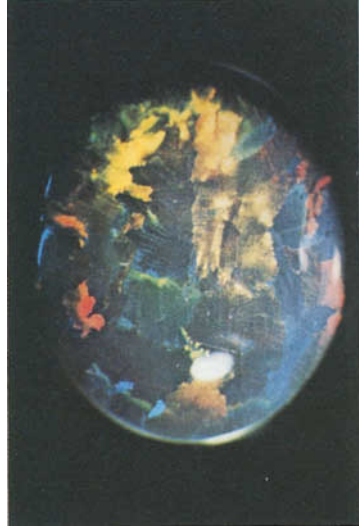
FIG. 12. Synthetic black opal (Gilson, Dec. 1975) showing mosaic with distinctly crenulate boundaries and "lizard skin" effect. \times 4 , reflected light.
