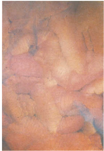
FIG. 4. Synthetic white opal (Gilson, Nov. 1974) showing "dendritic" line structure or "healed-scar" effect. \times 13 , transmitted light.
