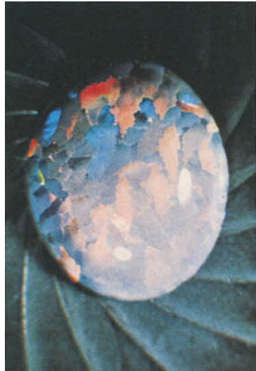
FIG. 14. Synthetic black opal (Gilson, Dec. 1975) showing "lizard skin" effect and crenulate margins. \times 12 , reflected light.
