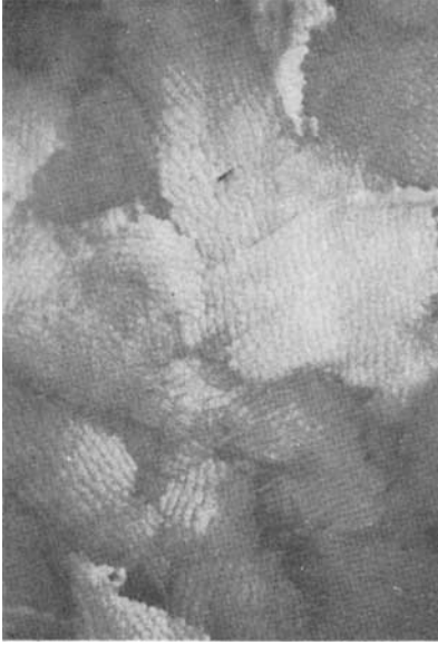
FIG. 7. Synthetic white opal (Gilson, Nov. 1975) showing "lizard skin" effect. \times 12 , transmitted light.
