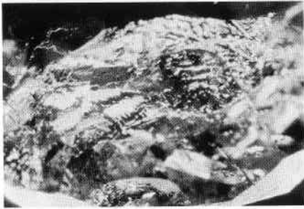
Figure 3. Liquid feathers interspersed with cleavage and tension cracks impairing the transparency of a faceted scorodite. 32x.
