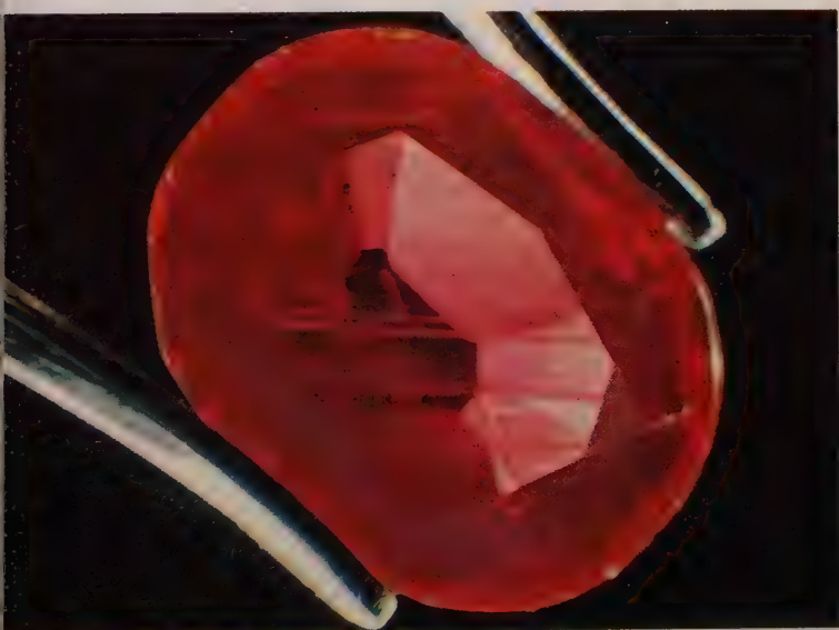
Ruby doublet showing straight bands in natural crown, and curved bands in synthetic base.
