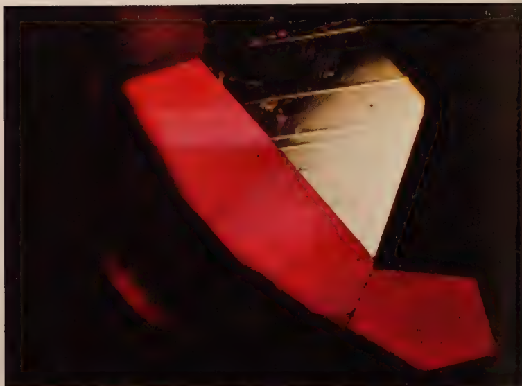
Siam ruby showing twin planes by transmitted light and their outcrop at the reflected surface.
