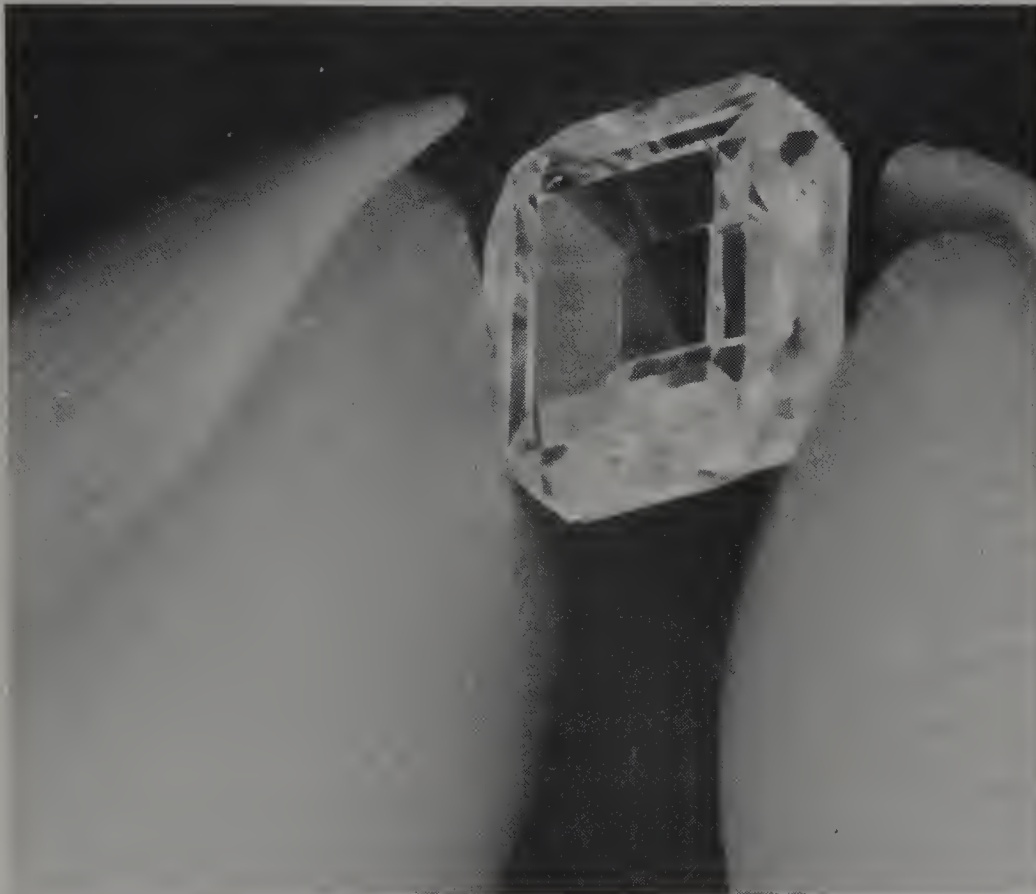
Figure 17.2. A gem quality synthetic diamond made by the General Electric Company of America
