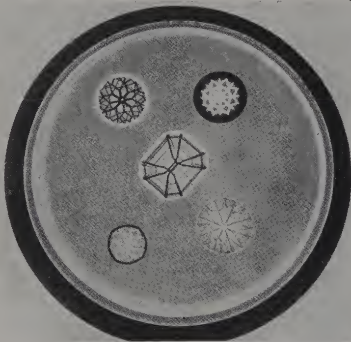
Figure 31.17. The effect of immersion contrast
