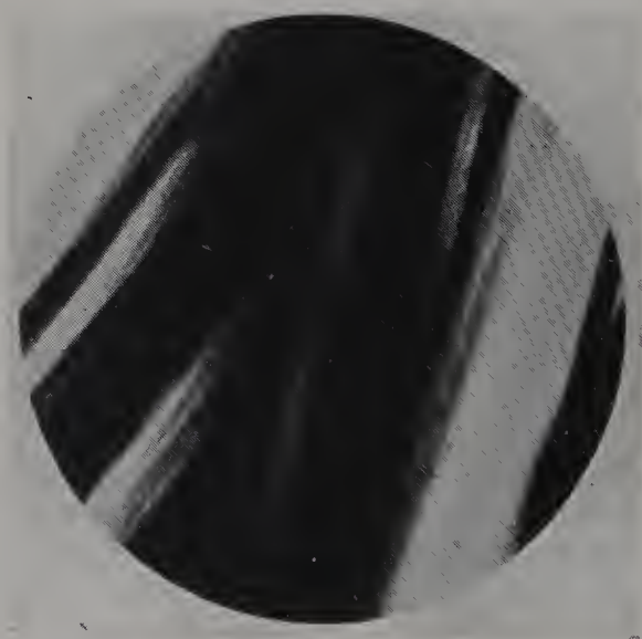
Figure 24.14. The colour in plastic imitations of tortoise-shell is in swathes
