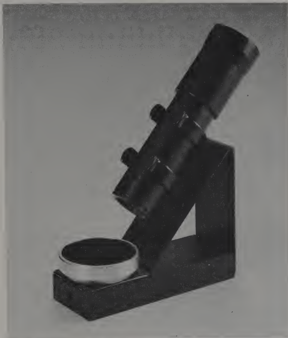
Figure 32.14. The new Rayner spectroscope with a series of slits of different widths which are put into the position by turning the eyepiece. The instrument as shown is held on a Mitchell type stand for reflected light observation. The diameter of the instrument allows it to be slipped into the body tube of a standard microscope in place of the ocular
