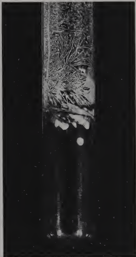
Figure 11.1. Feathery crystals of phthalic anhydride produced when alkyd resins are heated in a test tube
