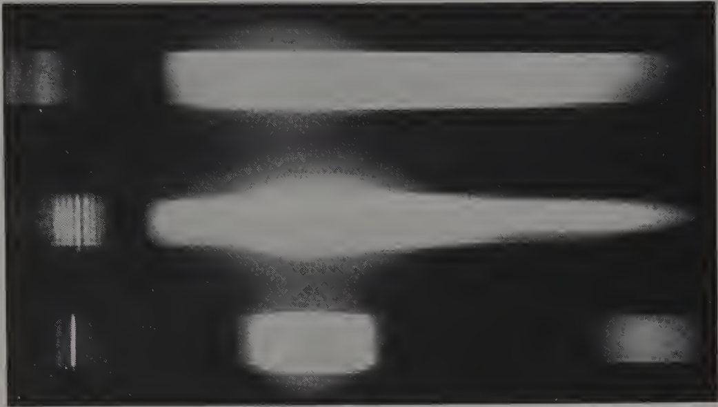
Figure 35.15. Fluorescence spectra of synthetic emerald (top), natural red spinel (centre), and ruby (bottom), excited by photoflood lamp and filtered through weak copper sulphate solution (By courtesy of B. W. Anderson)
