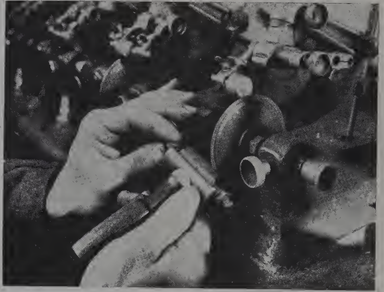
Figure 20.30. Charging the sawing disc with diamond powder
