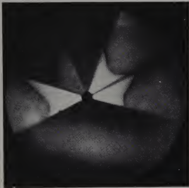
Figure 30.4. The 'umbrella' seen around the culet in a bottom-treated cyclotroned diamond
