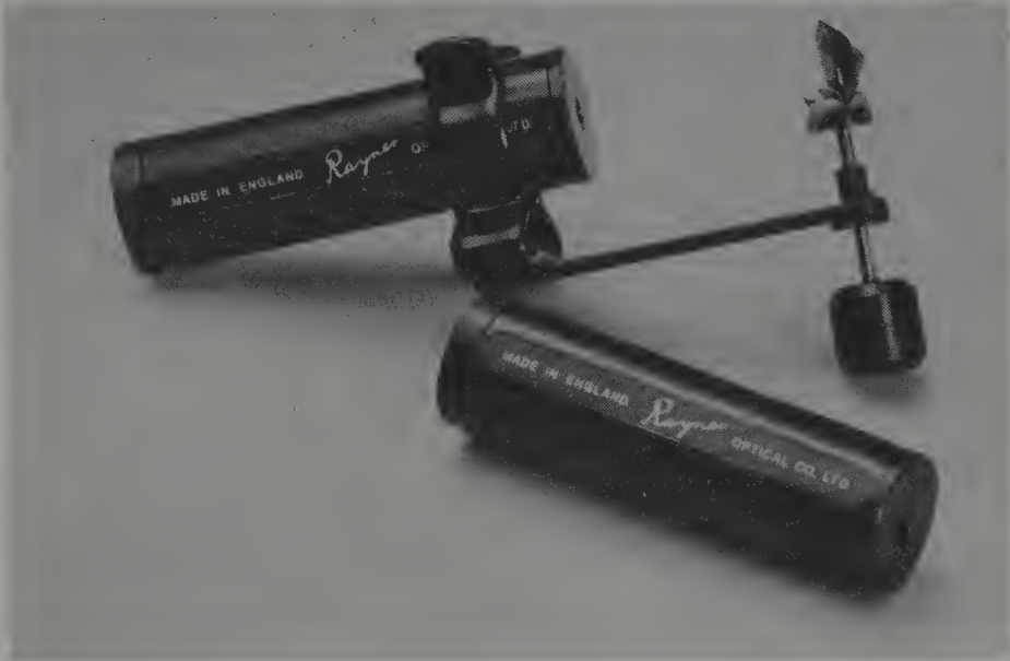
Figure 32.5. Dichroscope by Rayner with arrangement for holding the stone during observation of dichroism
