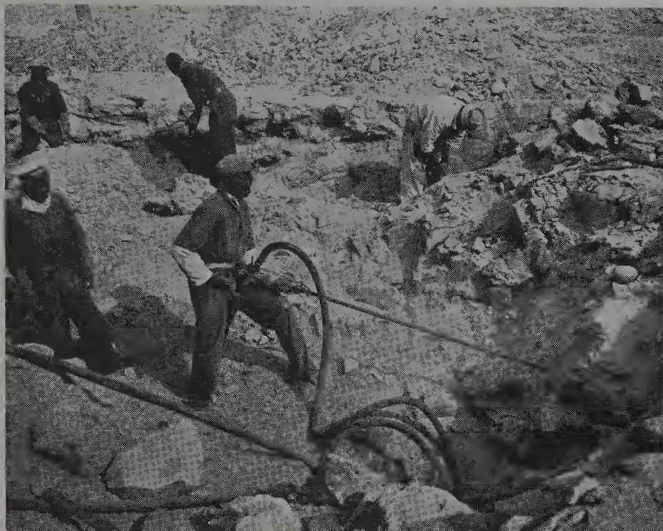
Figure 2.12. A native miner drills a hole into diamondiferous conglomerate in a mining face at Mittag preparatory to blasting (By courtesy of the Anglo-American Corporation of South Africa Ltd.)
