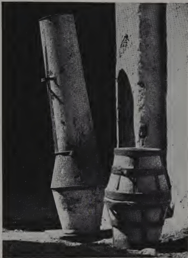
Figure 7.2. Heating rough zircon. Left, a tall funnel filled with coal. Right, one kilogram of rough zircon being heated
