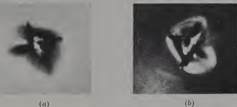
Figure 33.59. Zircon crystal surrounded with a halo in a Ceylon sapphire: (a) in transmitted light, (b) in dark-ground illumination
