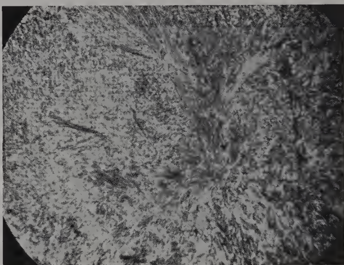
Figure 12.1. A photomicrograph of a thin section of nephrite showing the felted mass of fibrous crystals
