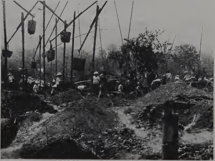
Figure 3.6. Washing the byon in the Burma ruby mines (By courtesy of the Editor, Journal of Gemmology )
