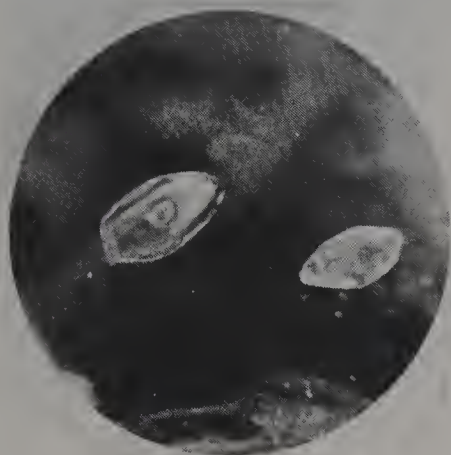
Figure 34.8. Negative crystals in a Ceylon sapphire. A typical example of primary auto-genetic inclusions
