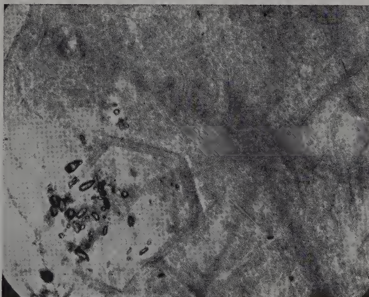
Figure 8.8. Characteristic 'eroded' crystals, probably in this case of zircon, and the peculiar oily streaks often called 'treacle' seen in a hessonite garnet
