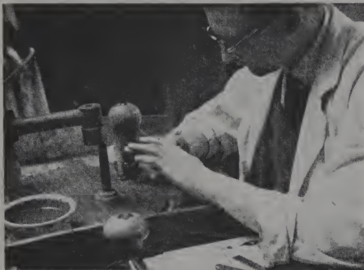
Figure 20.39. The lapidary's cutting lap showing the 'jamb peg' behind the lapidary's hand and the hand crank for driving the 'mill' in the foreground
