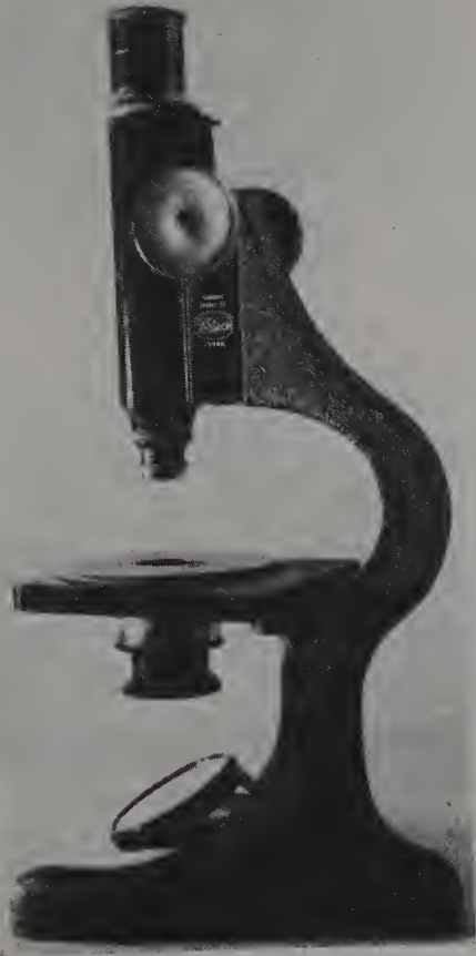
Figure 33.23. A simple fixed-stand microscope (the Beck, London No. 10) fitted with polarizing equipment and an extemporized rotating stage
