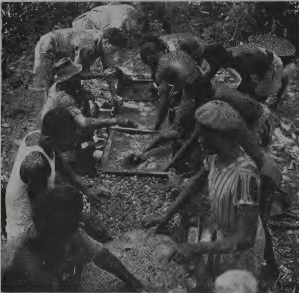
Figure 2.17. Natives grading the diamond-bearing gravel after it has been through the joplin jigs preparatory to the pebbles being searched for diamonds
