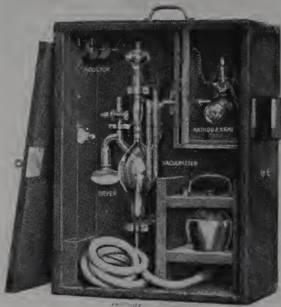
Figure 35.14. The complete unit for the production of cathode rays and x-rays as made by C. L. Herz of Vienna
