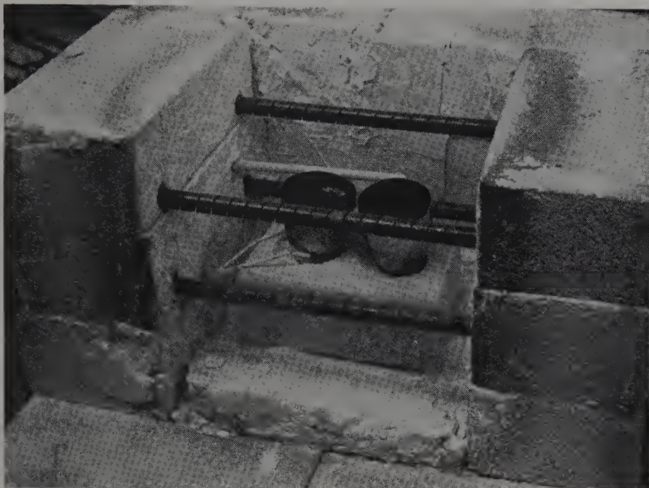
Figure 17.13. A flux-melt furnace used for the experimental production of synthetic stones
