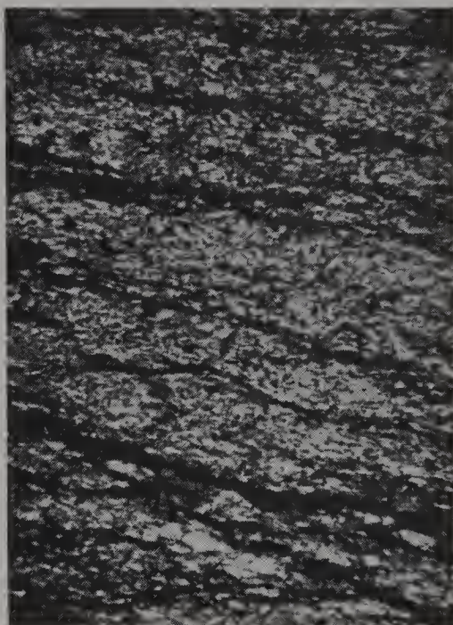
Figure 12.3. Photomicrograph of a thin section of jadeite showing the granular nature of this jade
