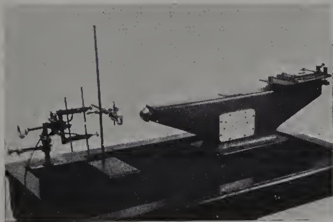
Figure 32.9. A quartz spectrograph set up for spectrum analysis
