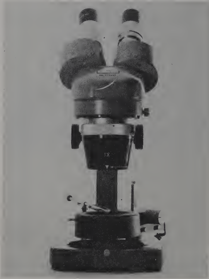
Figure 2.21. A microscope with dark-field illumination for use in diamond examination (By Eickhorst of Hamburg)
