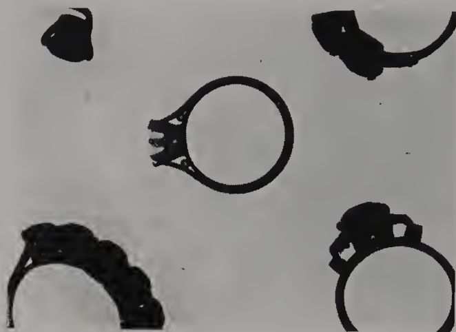
Figure 2.29. A radiograph of a diamond ring (centre), two zircon rings, a tie pin and a 5-stone synthetic rutile ring showing the difference in transparency of the diamond
