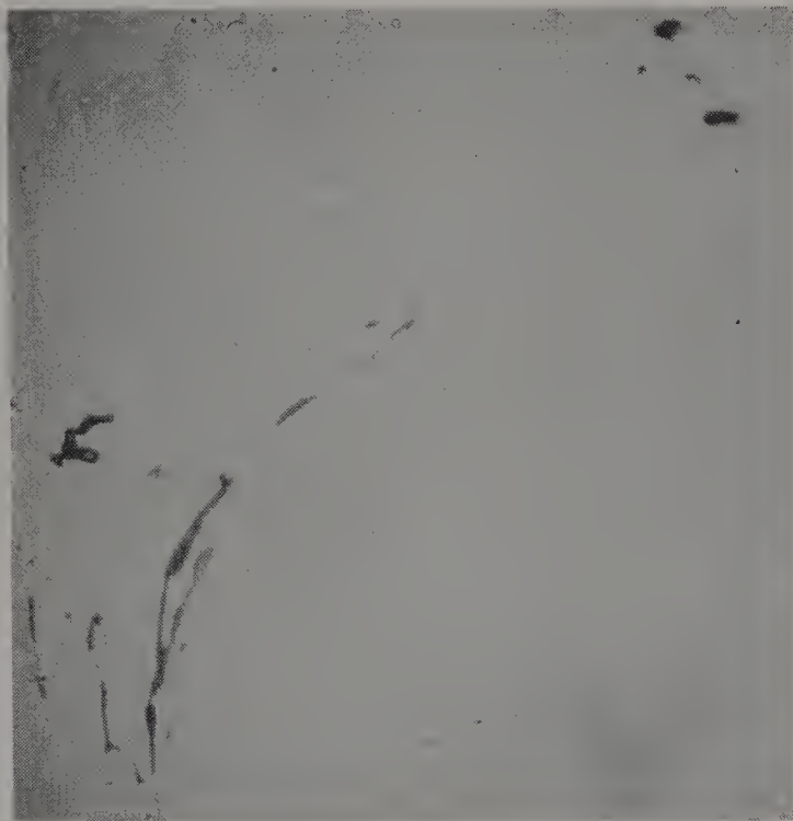
Figure 17.35. Inclusions in a 'pulled' crystal of yttrium aluminate
