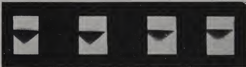
Figure 36.12. Radiographs of a diamond doublet. Diamond top and synthetic white sapphire base. These are four different exposures
