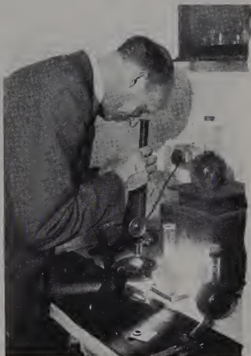
Figure 32.16. Using the spectroscop by the microscope method
