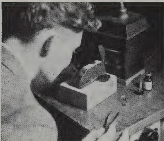
Figure 32.11 Observing the shadow edge with the refractometer (the lid has been left up for photographic purposes)
