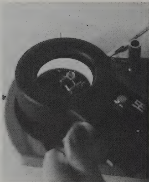
Figure 34.39 Adjustable 'ring' light for open or microscope stage use which will give incident or dark-field illumination
