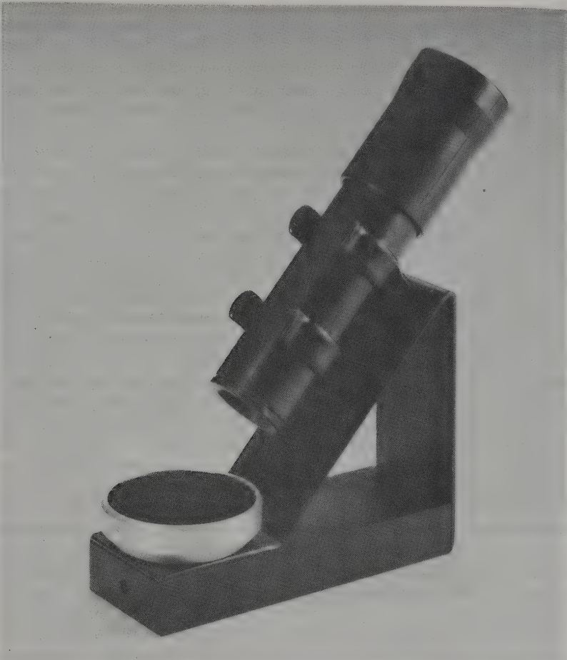
Figure 33.14 The Rayner direct-vision diffraction spectroscope with a series of slits of different widths which are put into the position by turning the eyepiece. The instrument as shown is held on a Mitchell stand for reflected light observation. The diameter of the instrument allows it to fit into the body tube of a standard microscope in place of the ocular
