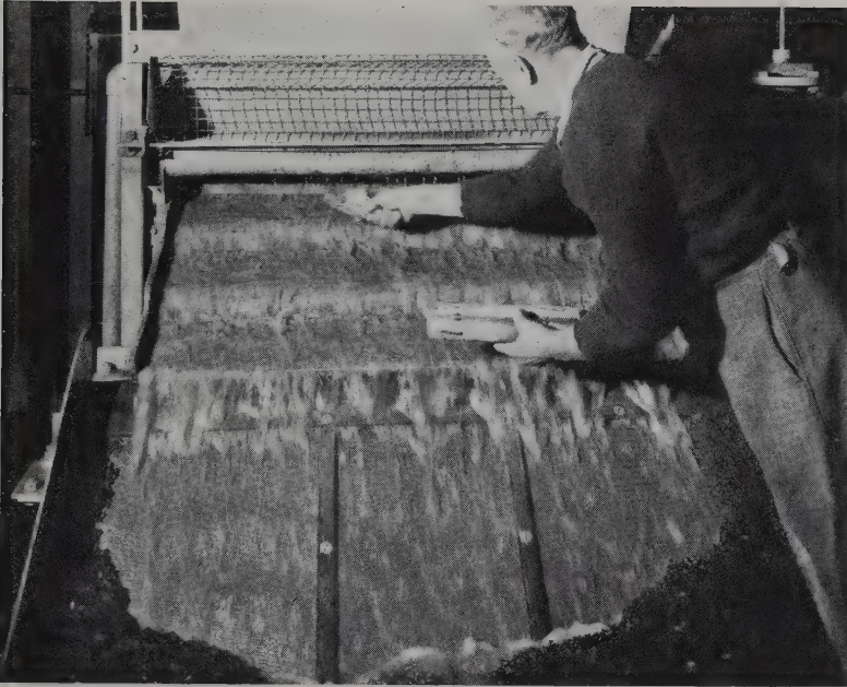
Figure 2.13 Removing diamonds from the grease table at Kimberley (by courtesy of the Anglo-American Corporation of South Africa Ltd)
