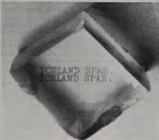
Figure 30.14 The doubling of print as seen through a rhomb of Iceland spar
