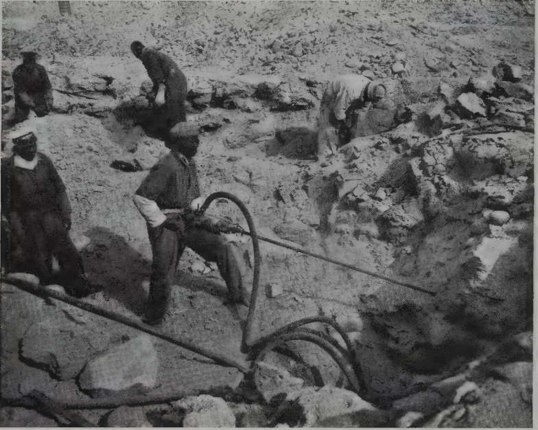
Figure 2.16 A miner drills a hole into diamondiferous conglomerate in a mining face at Mittleage preparatory to blasting (by courtesy of the Anglo-American Corporation of South Africa Ltd)
