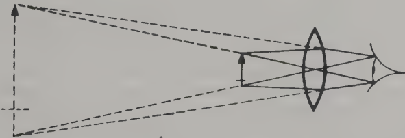
Figure 34.4 The formation of a virtual image by a convex lens. The principle of the magnifying glass
