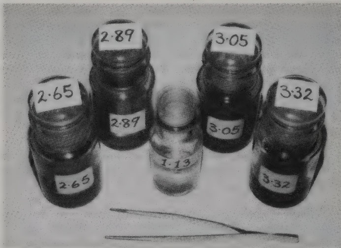
Figure 29.1 A set of heavy liquids: the smaller bottle contains a salt solution for checking amber (see Chapter 24)
