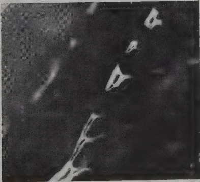
Figure 34.64 Photomicrograph taken on bromide paper of two-phase inclusions in a white topaz
