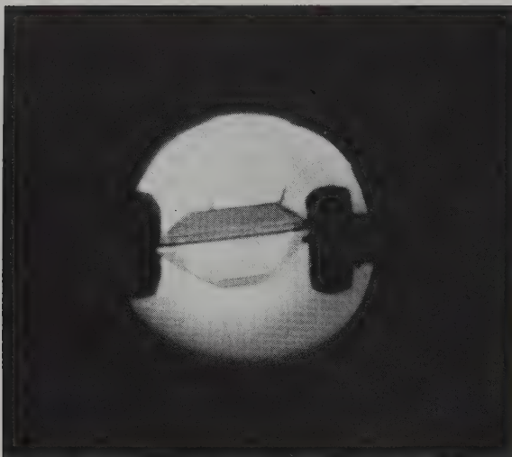
Figure 20.5 A spinel souldé emerald immersed in di-iodomethane and viewed through the side clearly shows the colourless top and bottom and the line of green colour
