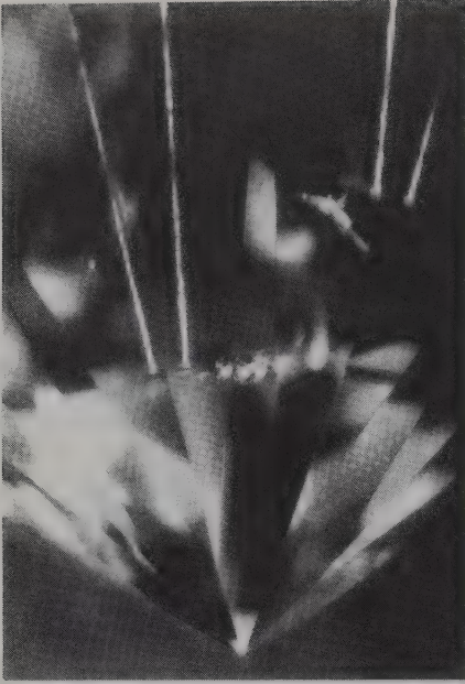
Figure 2.23 Two laser drill holes (reflected between facets) reaching inclusions within a diamond (courtesy GIA)
