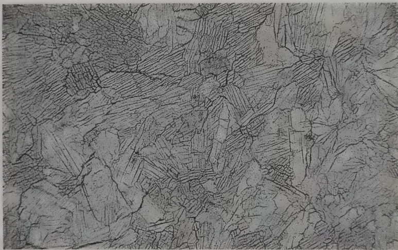
Figure 13.3 Photomicrograph of a thin section of jadeite showing the interlocking granular texture (Myanmar specimen under plane polarised light)
