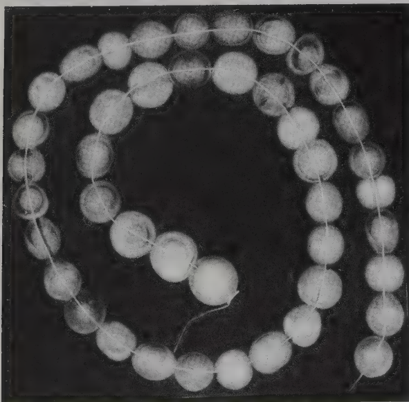
Figure 22.37 Direct X-ray picture of a natural pearl necklet (negative image of positive print)
