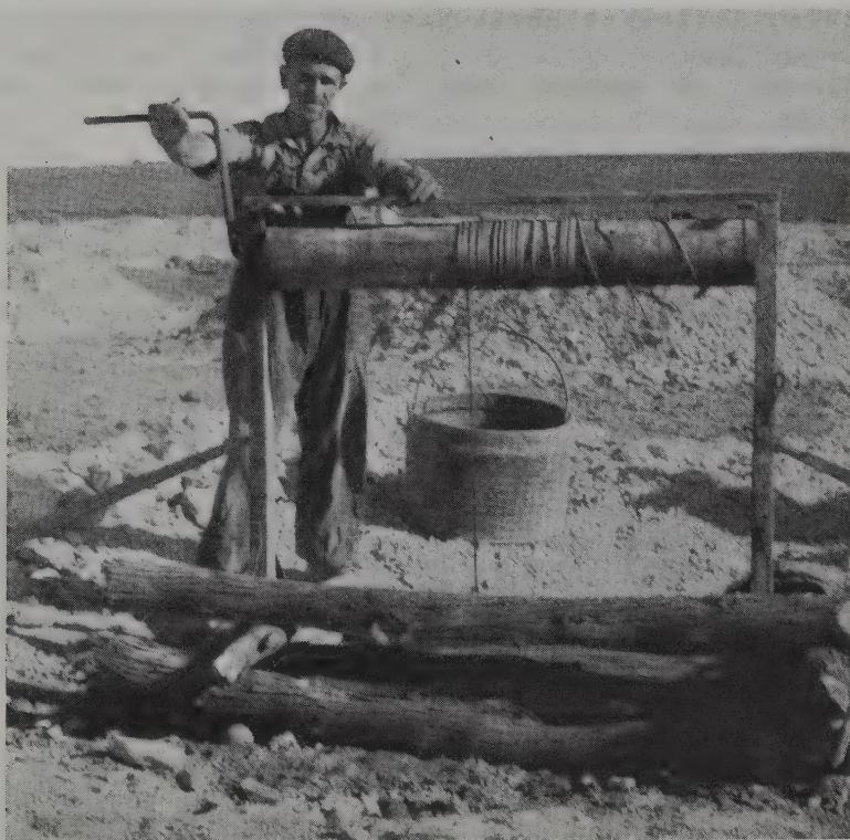
Figure 11.3 Opal mining at Andamooka. The miner turning the windlass is hauling up a bucket which a miner below ground has filled
