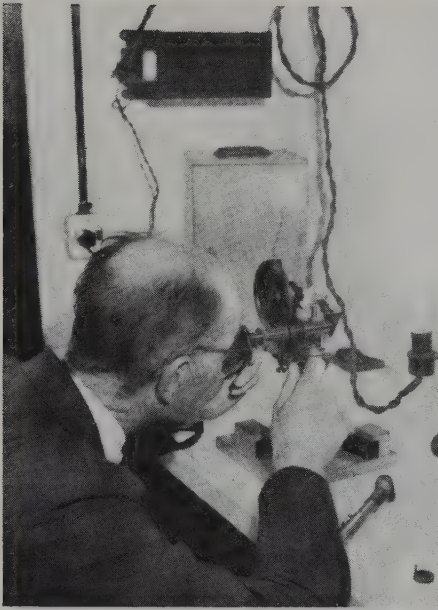
Figure 32.1 The Abbe-Pulfrich refractometer in use
