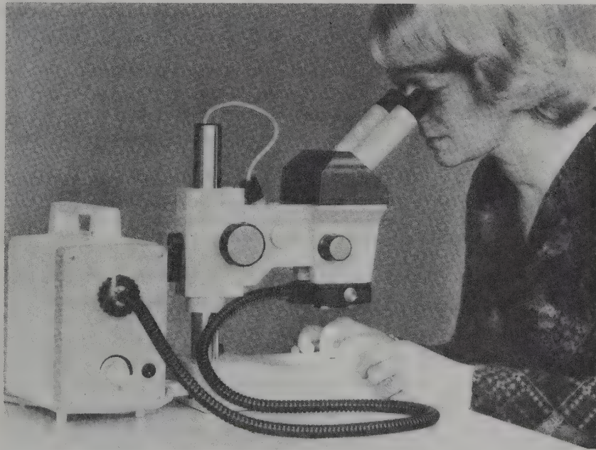
Figure 34.29 The light source KL 1508, shown fitted to a special microscope light guide which gives shadowless incident illumination (Schott)
