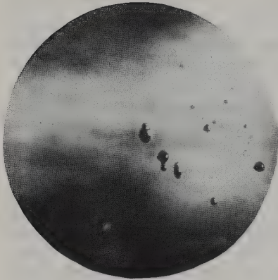
Figure 34.44 'Tabby extinction' and 'profilated' gas bubbles in a synthetic spinel
