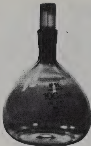
Figure 29.3 The pycnometer or specific gravity bottle
