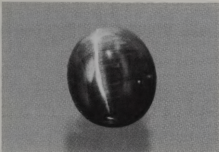
Figure 6.21 Cat's-eye tourmaline containing parallel hollow tubes (photo by Maha DeMaggio, Gemological Institute of America)
