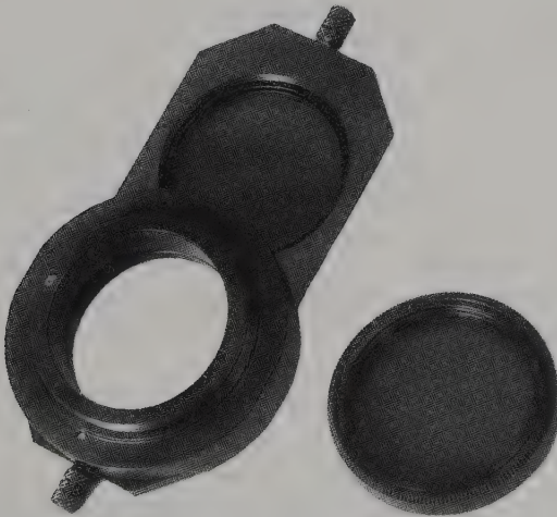
Figure 34.25 Auxiliary polarising equipment showing a Polaroid polariser that fits on the stage of the microscope below the subject, and an analyser designed for rotation that fits just below the objective lens and above the subject
