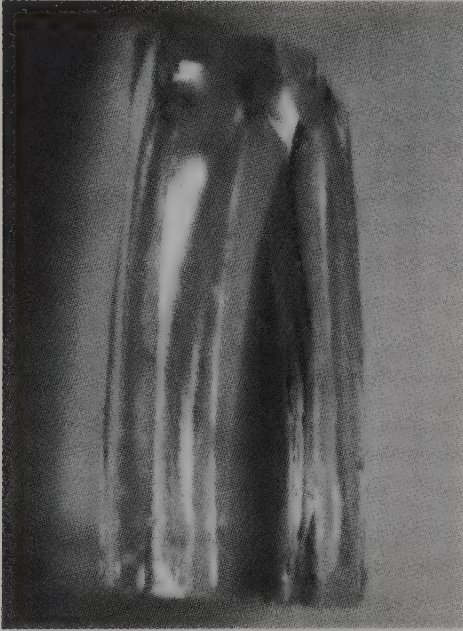
Figure 18.40 A single crystal of cubic zirconium oxide (weighing around 600 carats) as broken out of the mass of crystals in the skull crucible
