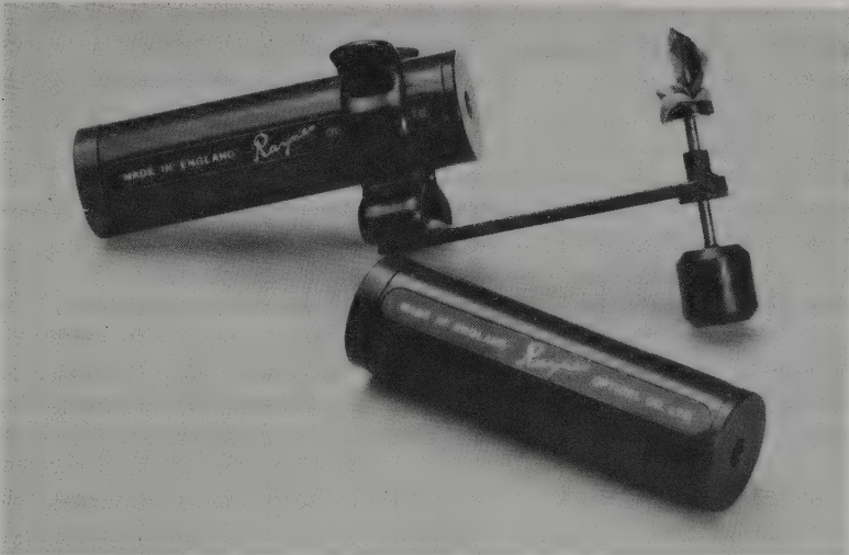
Figure 33.5 Dichroscope by Rayner with arrangement for holding the stone during observation of dichroism
