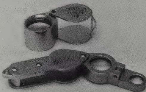
Figure 34.8 Krüss hand loupes; the lower one has a hinged supplementary lens giving a choice of magnifying powers
