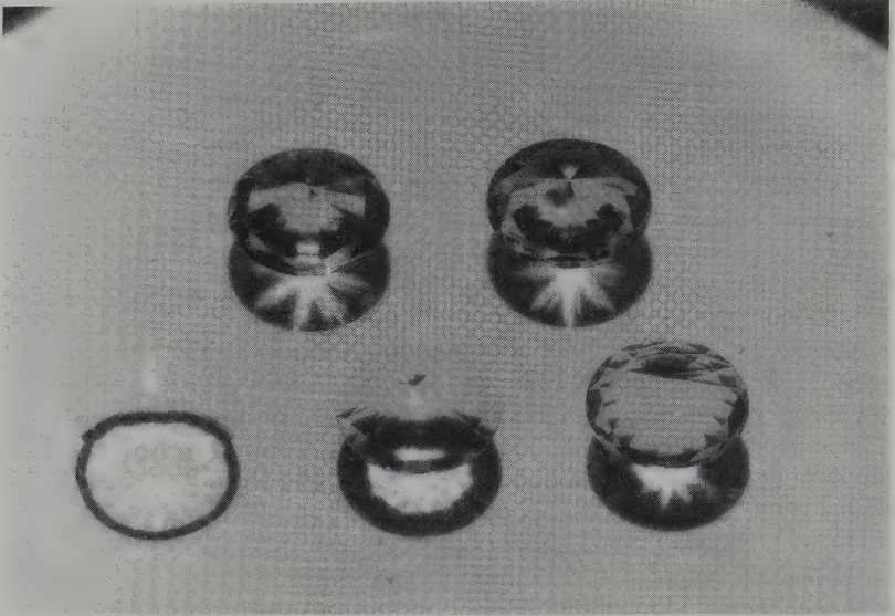
Figure 2.37 When light is placed over stones immersed in di-iodomethane (methylene iodide), different stones show differing patterns: top row (left to right) strontium titanate, diamond, bottom row YAG, GGG, CZ (Courtesy GIA)
