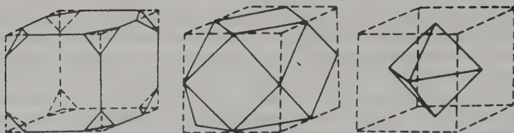
Figure 28.1 The cleavage directions of fluor spar, showing how an octahedral form can be cleaved out of a cube crystal
