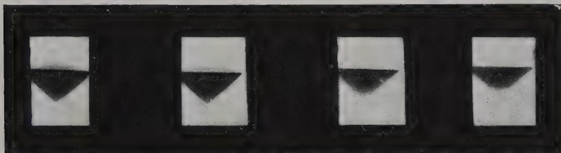
Figure 37.6 Radiographs of a diamond doublet. Diamond top and synthetic white sapphire base. These are four different exposures
