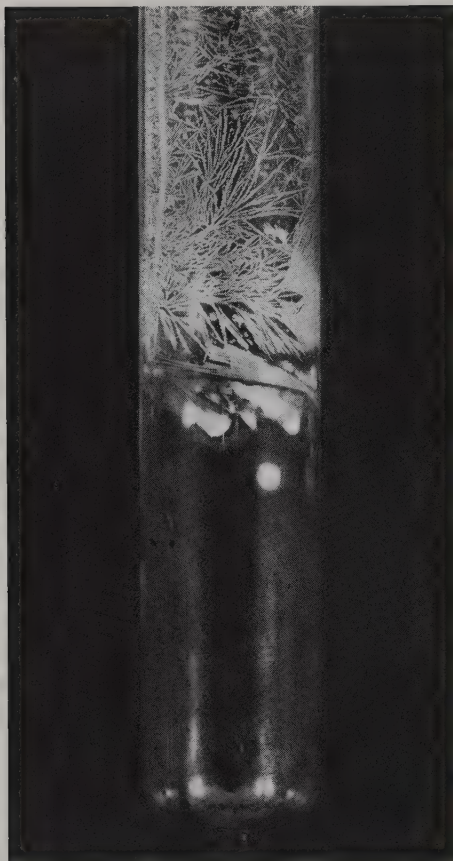
Figure 12.1 Feathery crystals of phthalic anhydride produced when alkyd resins are heated in a test tube (photo: G Wild)
