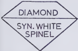
Schematic drawing of a semi-genuine doublet (in this case a diamond doublet).
