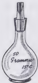
FIG. 18.—The pycnometer or "specific gravity bottle."
