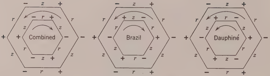
FIG. 46. Diagrams illustrating the relation between the axial systems and hand of crystals twinned on the three parallel-axes laws. Arrows indicate hand.
