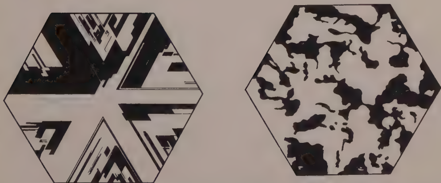
FIG. 48. Etched basal sections of quartz, showing mosaic type of Dauphiné twinning (right) and Brazil twinning (left). Leydolt, 1855.
