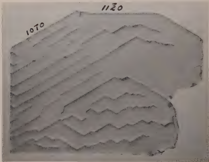
FIG. 72. (0001) section of quartz containing cleavage cracks on (10\bar{1}0) produced by thermal shock.
