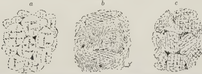
a, Serpentine derived from chrysolite; b, from amphibole; c, from pyroxene
