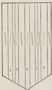
Plagioclase with twinning lamellæ. Fig. 815 section \parallel c(001) showing vibration-directions (cf. Fig. 819), ordinary light; Fig. 816 section in polarized light.
