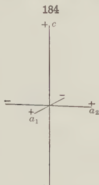
Axes of Tetragonal Mineral, Octahedrite a : c = 1 : 1.78
