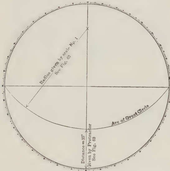
Location of the arc of a great circle in the Stereographic Projection at a given angle above the equator
