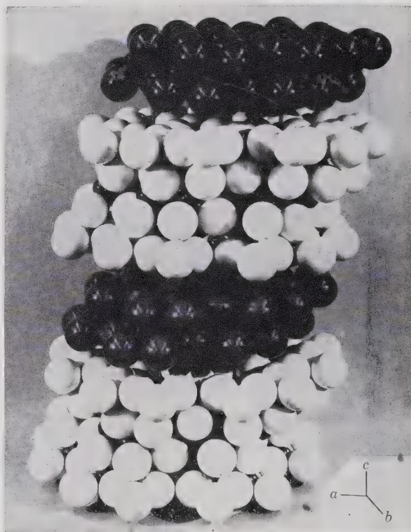
Fig. 594. Chlorite, \text{Mg}_3\text{Si}_4\text{O}_{10}(\text{OH})_2 \cdot \text{Mg}_3(\text{OH})_6 , Packing Model. O white, (OH) large black, Mg small black; c axis vertical. The model shows "t-o-t" sheets alternating with "o" sheets. Fe II , Fe III and Al may substitute for Mg and Al for Si.
