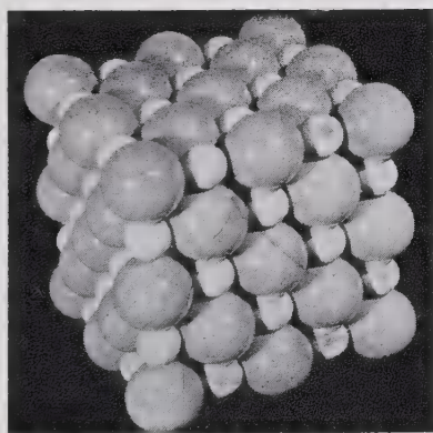
Fig. 466. Halite, \text{NaCl} , Packing Model. Na white, Cl gray.
