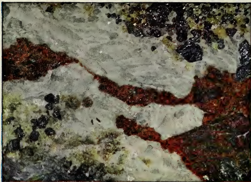
Specimen in White Light Showing White Calcite, Red Zincite, Pale Green Willemite and Blue-black Franklinite.
