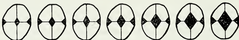
Fig. 542. Successive Cross Sections through a Chiastolite Crystal.
