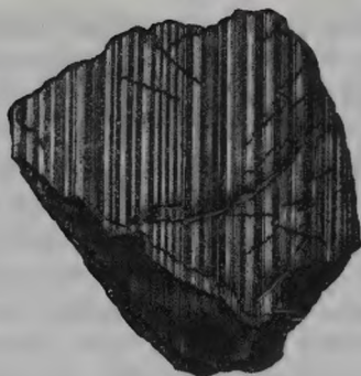
Striations appearing on {001} cleavage plane of polysynthetic twinning on the albite law.
