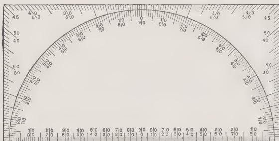
Stereographic Protractor for plotting Stereographic Projections (after Penfield; reduced one-half)
